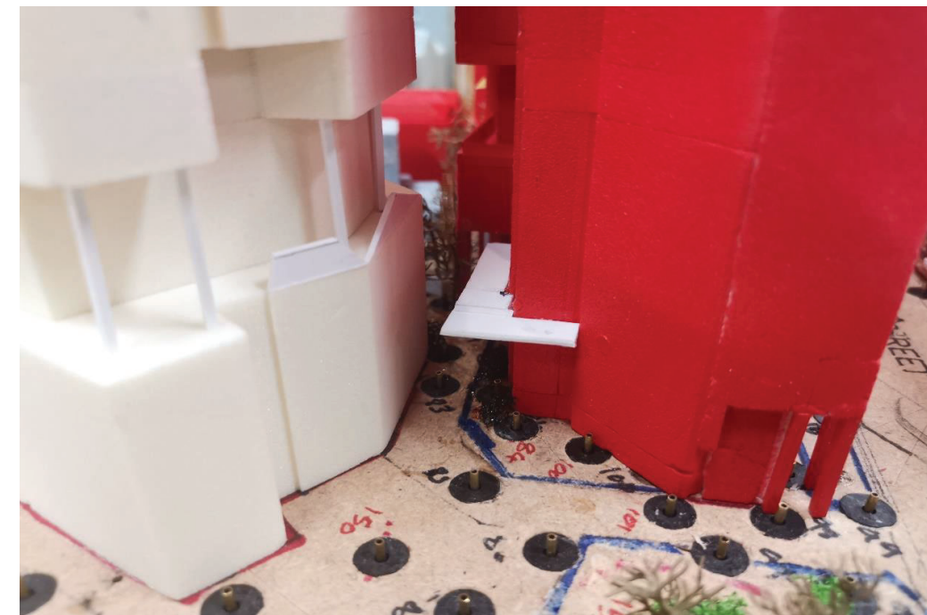
Figure 16: Wind Mitigation Measures (Configuration 6)
