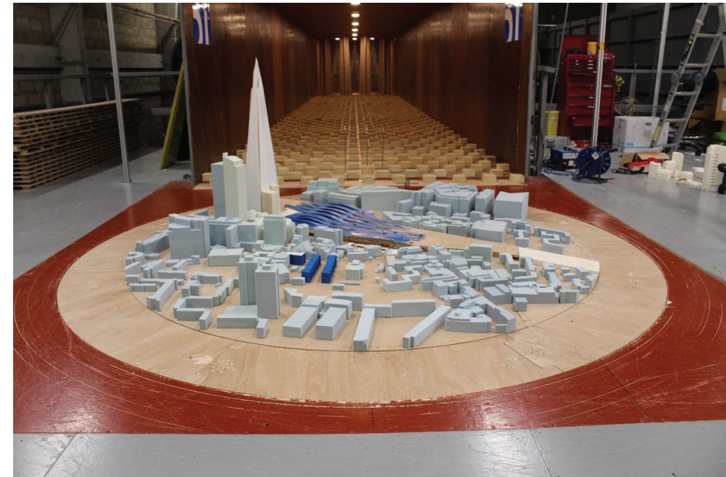
Figure 3: Existing Site with Existing Surrounding Buildings (Configuration 1) - View of the Model (from the south)
