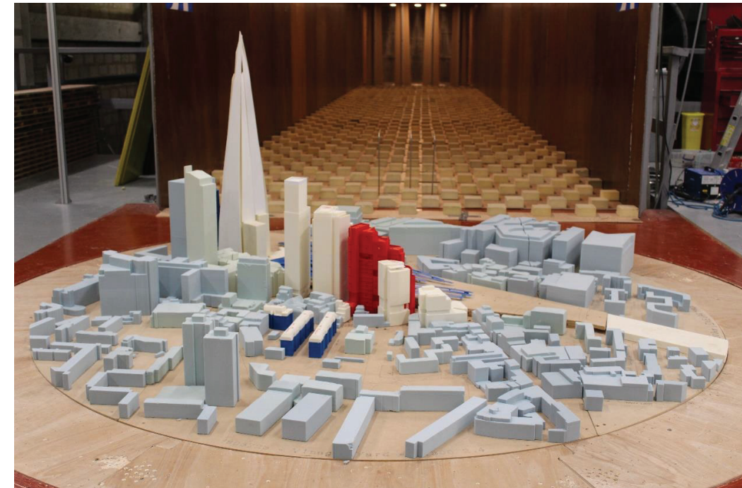
Figure 11: Proposed Development with Cumulative Existing Surrounding Buildings, Capital House, The Edge, and Sellar Scheme (Configuration 5) – View of the Model (from the south)
