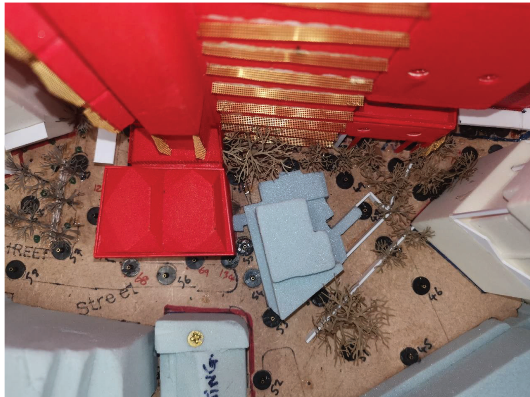
Figure 18: Wind Mitigation Measures (Configuration 6)
