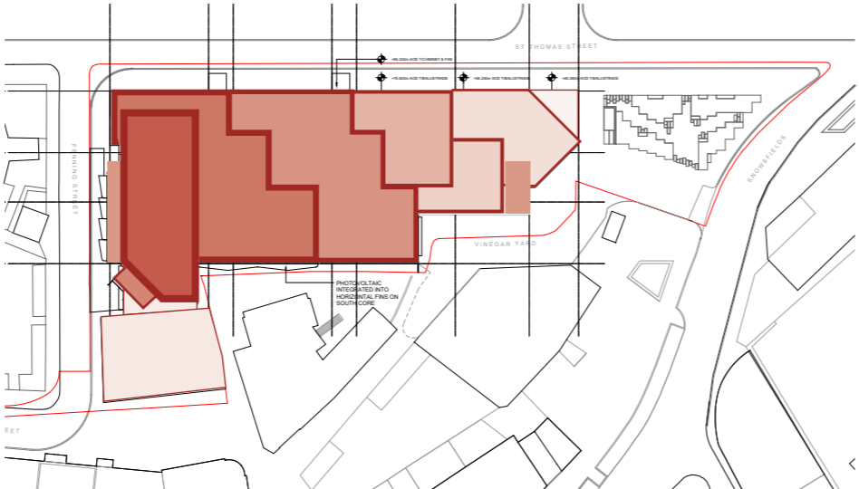
Height located on west of site to step down to Bermondsey Conservation Area
