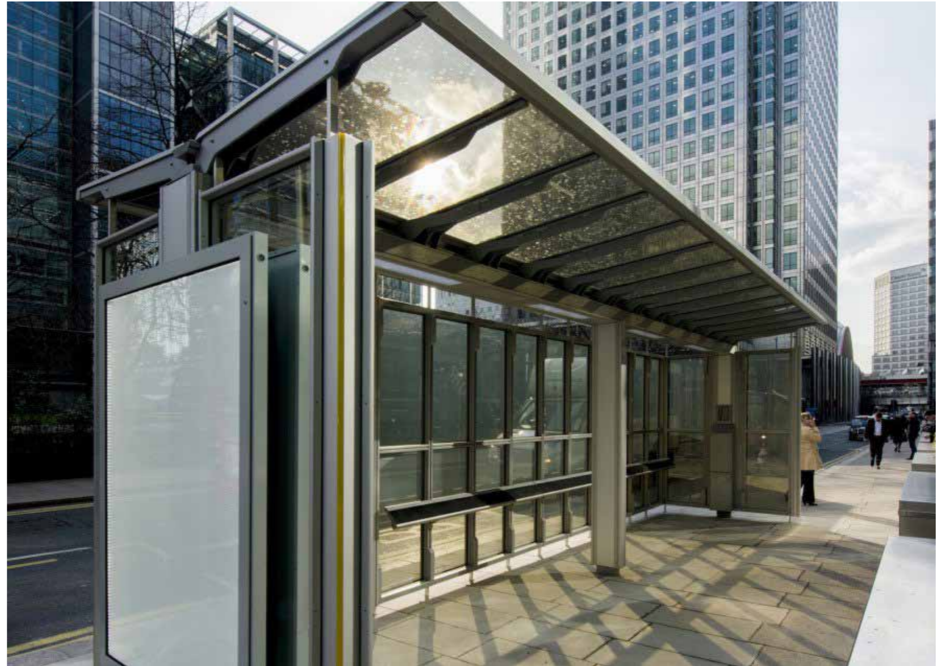
Example - Transparent Photovoltaic Glass Bus Shelter - Canary Wharf
