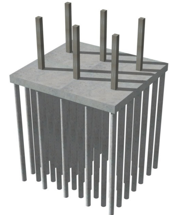
Figure 7.1 Typical piled raft solution
