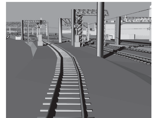
Fig. 06: Computer model of train tracks & signals from photogrammetry
