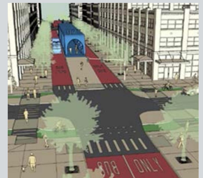
FIG 2.9 Concept drawing of a dedicated bus transit street through a new development
