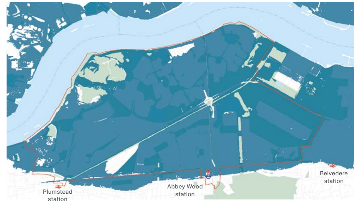
FIG 3.53 Areas at risk of flooding during an extreme flood event if flood defences were to breach or fail (Thames Tidal Breach Inundation, 2018)
