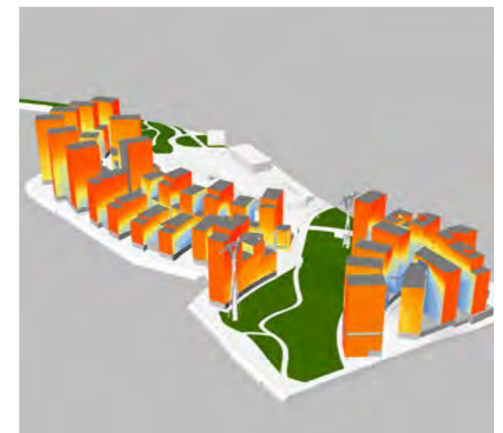
Solar exposure from overheating risk analysis (Red and Orange outlining risk mitigated areas)
