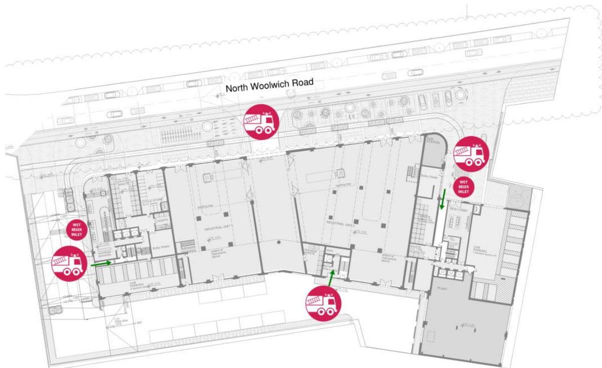
Figure 2: Indicative Fire Vehicle Parking Positions on site
