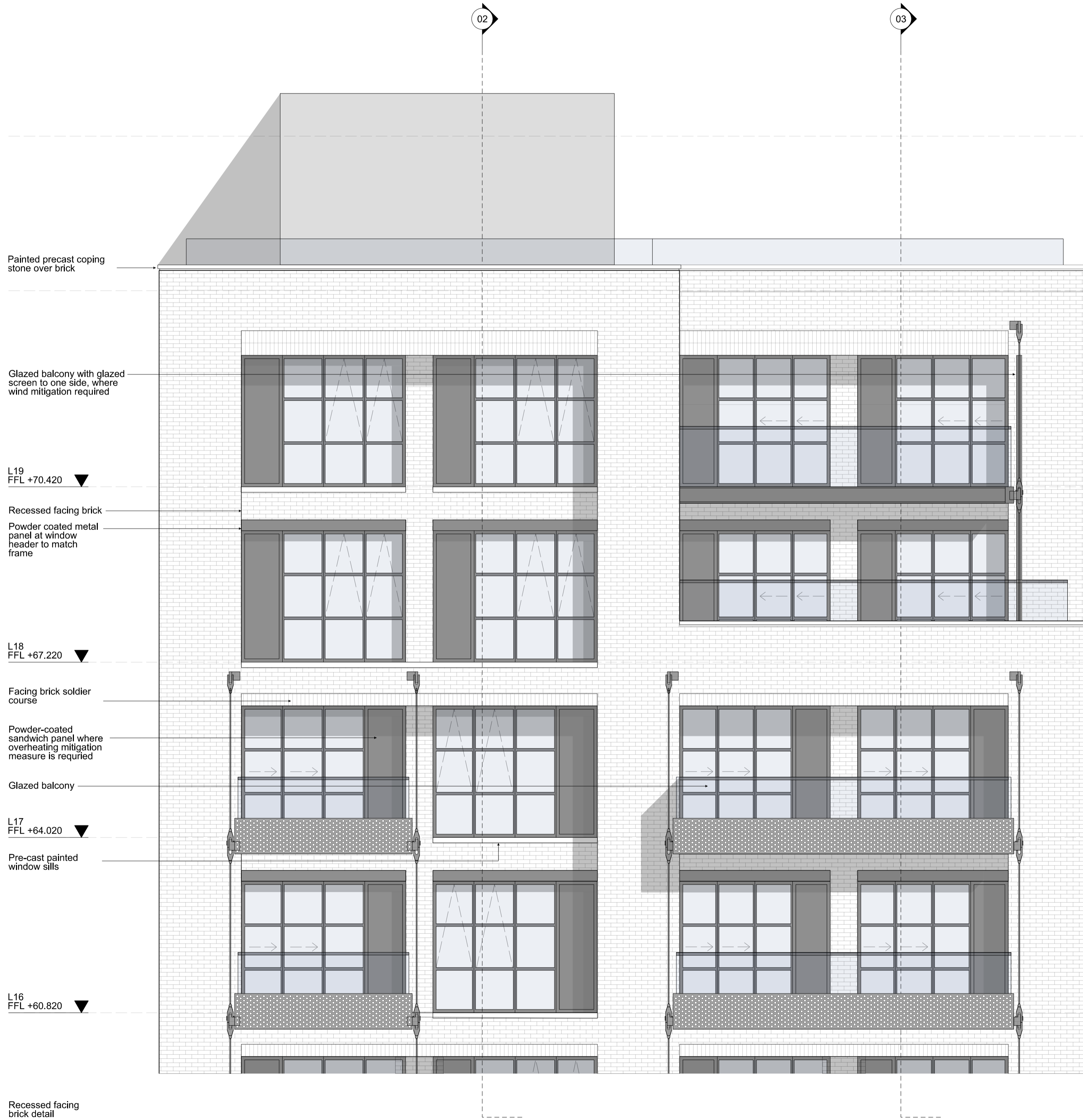
01 TYPICAL BAY 02 - ELEVATION 1:50
