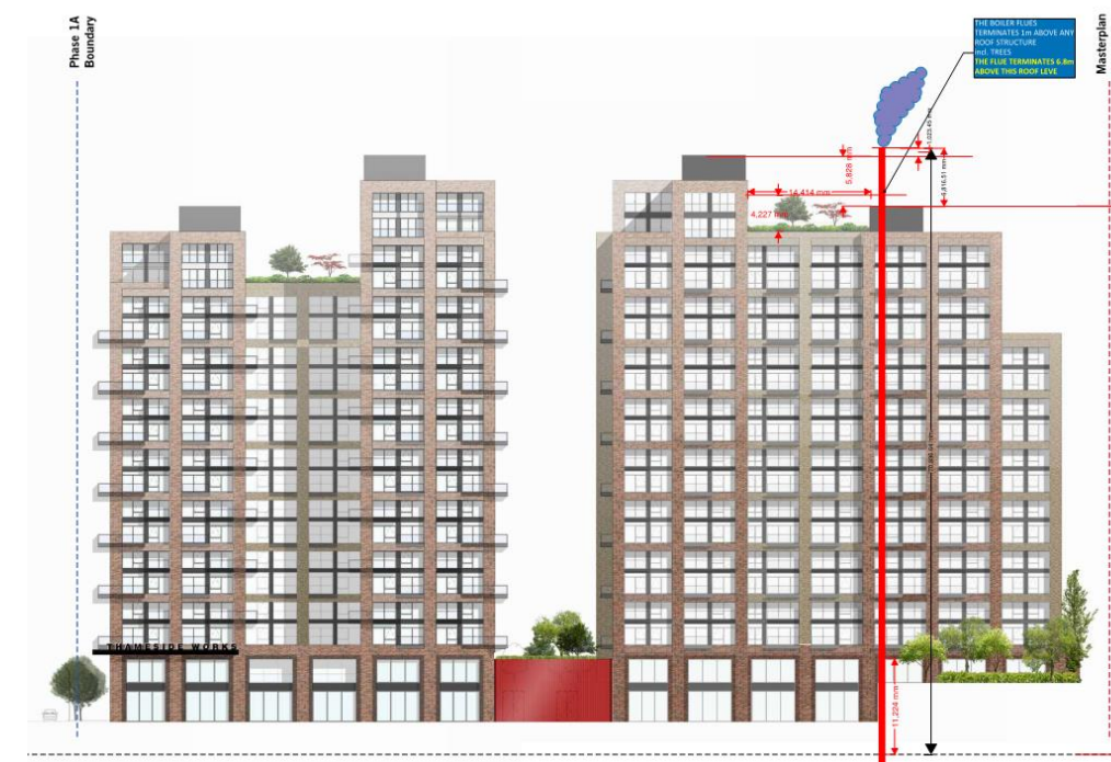
Figure 7-2 Previously located boiler flue
