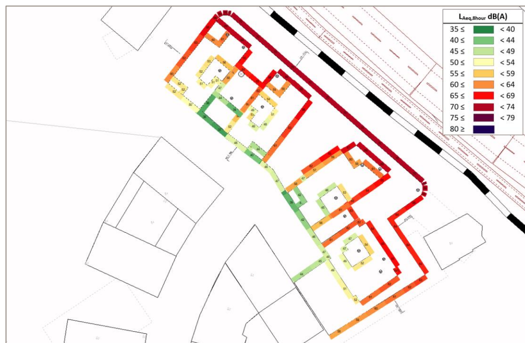
Figure 6—2 Predicted night-time ambient noise levels at 1 m from façade on Phase 1
