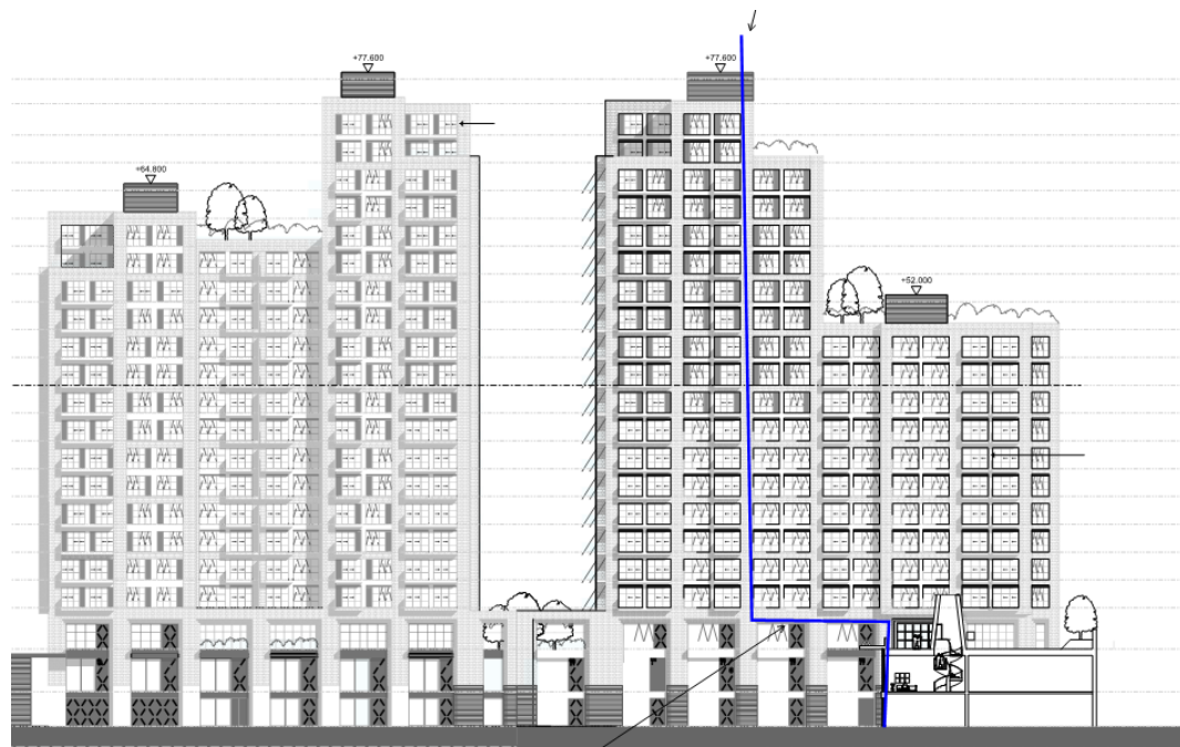
Figure 7-3 Diagram showing relocated flue termination (March 2020)
