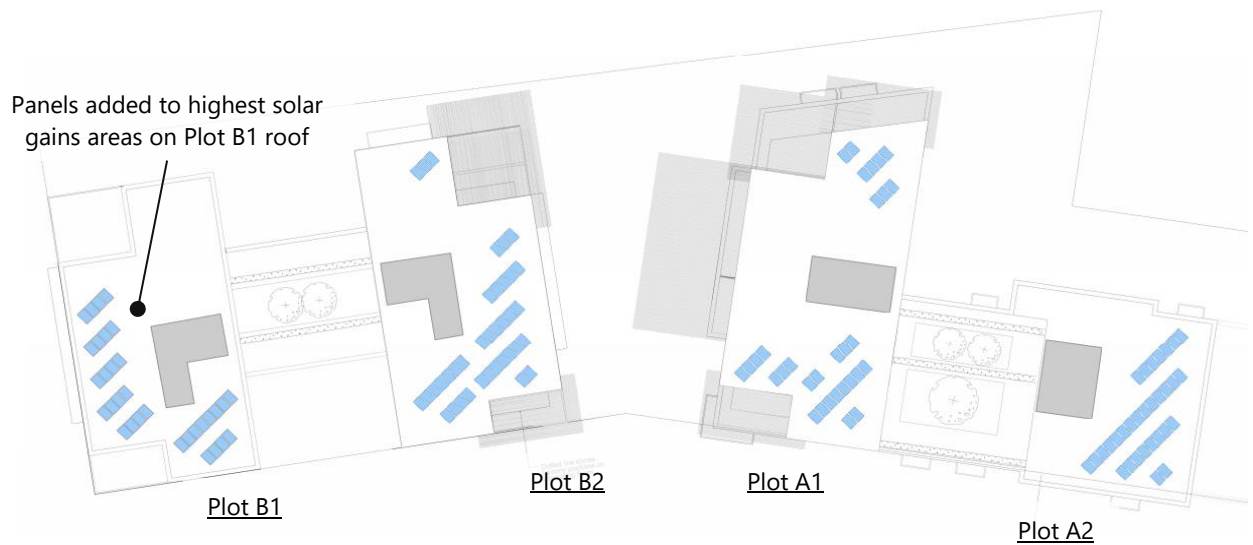
Figure 2—18 the detailed PV layout for the roofs of plots A and B as based on the optimisation
