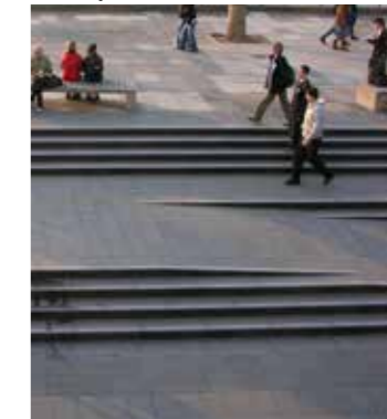
Stepped / ramped level changes
