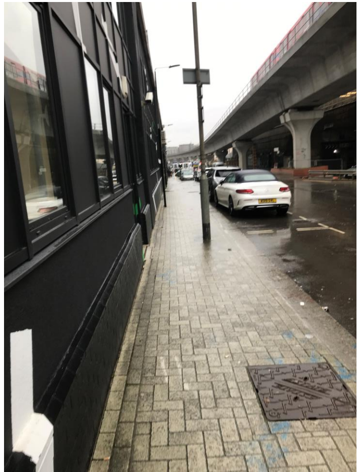
Lamp column placement restricts effective width significantly
