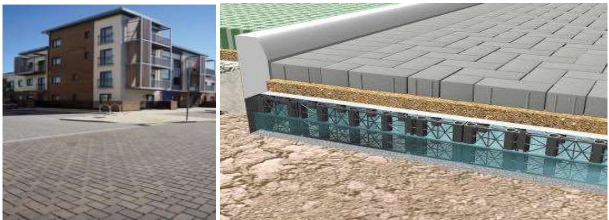
Figure 3: Typical podium attenuation details
