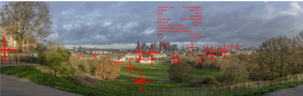
01.6 Screen grab of camera matching to survey data
