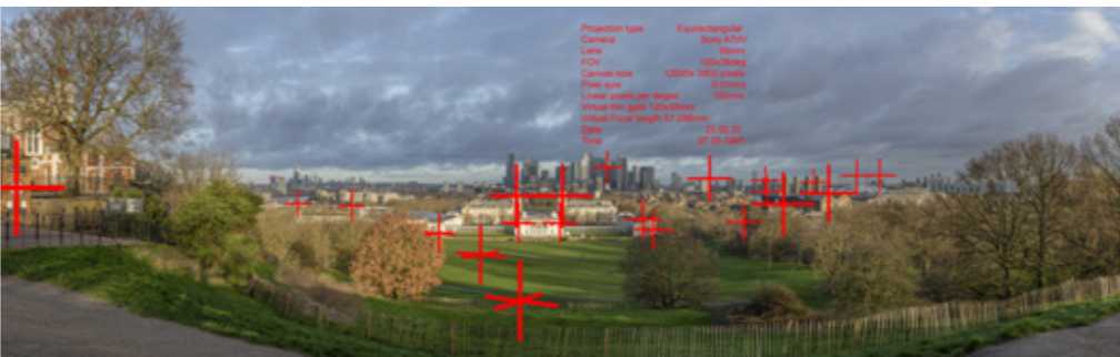
01.7 Screen grab of wireline model matched to photograph
