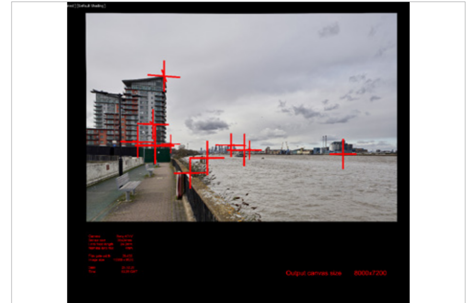
01.6 Screen grab of camera matching to survey data
