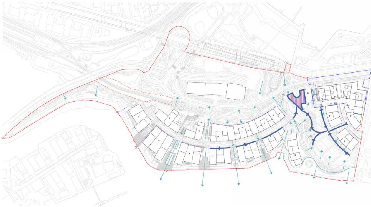
Figure 13—5 Masterplan Drainage and SUDs strategy diagram (small arrows shows falls, thick blue shows dry swales, pink shows reed bed/water feature)
