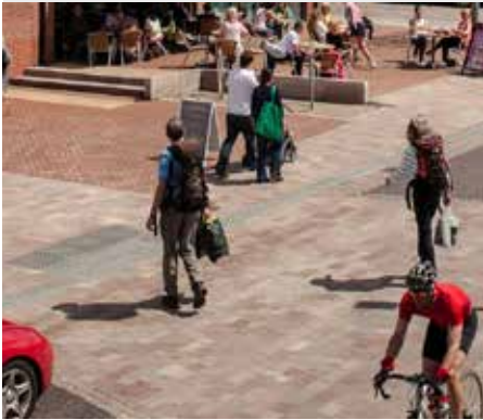
Paving change indicating pedestrian crossing
