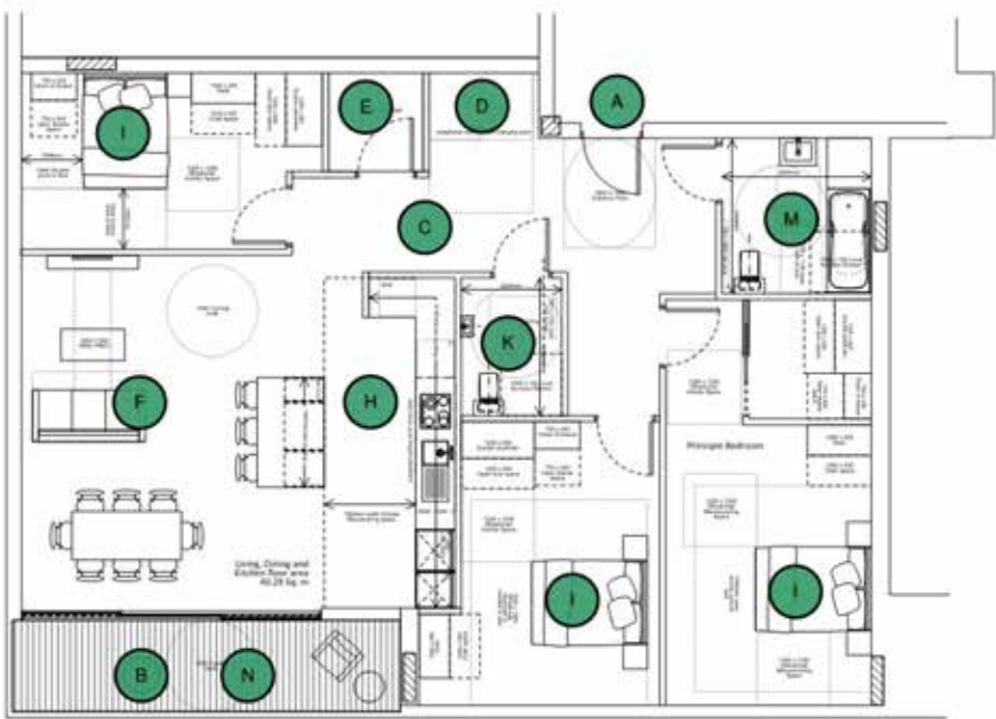
Fig 7.1.6 Typical unit conforming to the requirement of M4(3) 2b wheelchair accessible with indicative lettering
