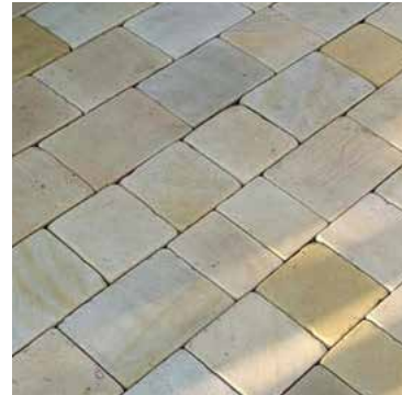
Surface Type 02 Yorkstone 'Scoutmoor' Setts Supplier: Marshalls Size: 100x100x80mm Finish: Diamond sawn
