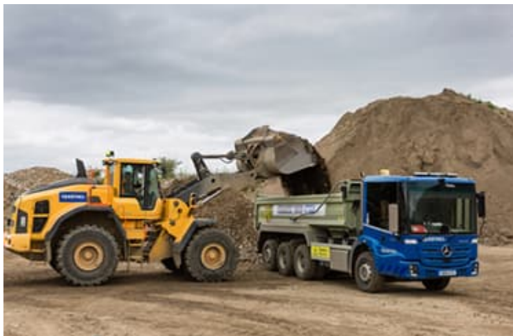
Figure 4-3 Example 32-Tonne Tipper Lorry
