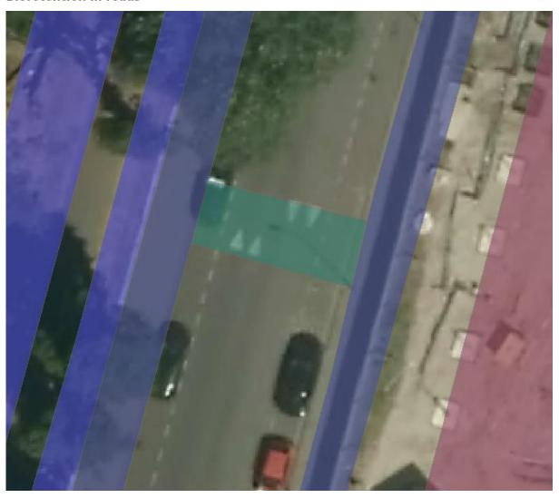
Bioretention solutions are landscaped planted depressions that drain surface water from all areas, except residential houses – which is where they mainly differ from rain gardens. Bioretention solutions include pocket infiltration, bioretention and multiple tree pits, with some storage capacity provided between the edge kerbs on roads.
