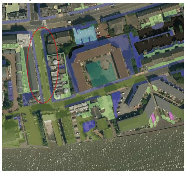
The only constraint for direct discharge to the Thames is that the run-off source must be within 15m of the river. In the example above the highlighted section of road is further than 15m from the river. However, since OS Mastermap considers this to be a single polygon attached to the riverside road, it has been flagged as having potential for direct drainage.
