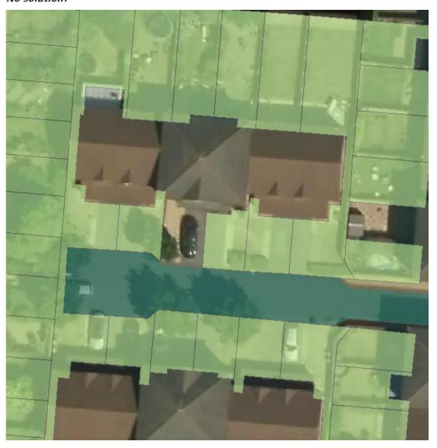
The above example shows a couple of garden polygons with no apparent SuDS solution. This could be perfectly valid since the expected run-off from surrounding sources might be managed sufficiently by using the surrounding rain garden sinks.
