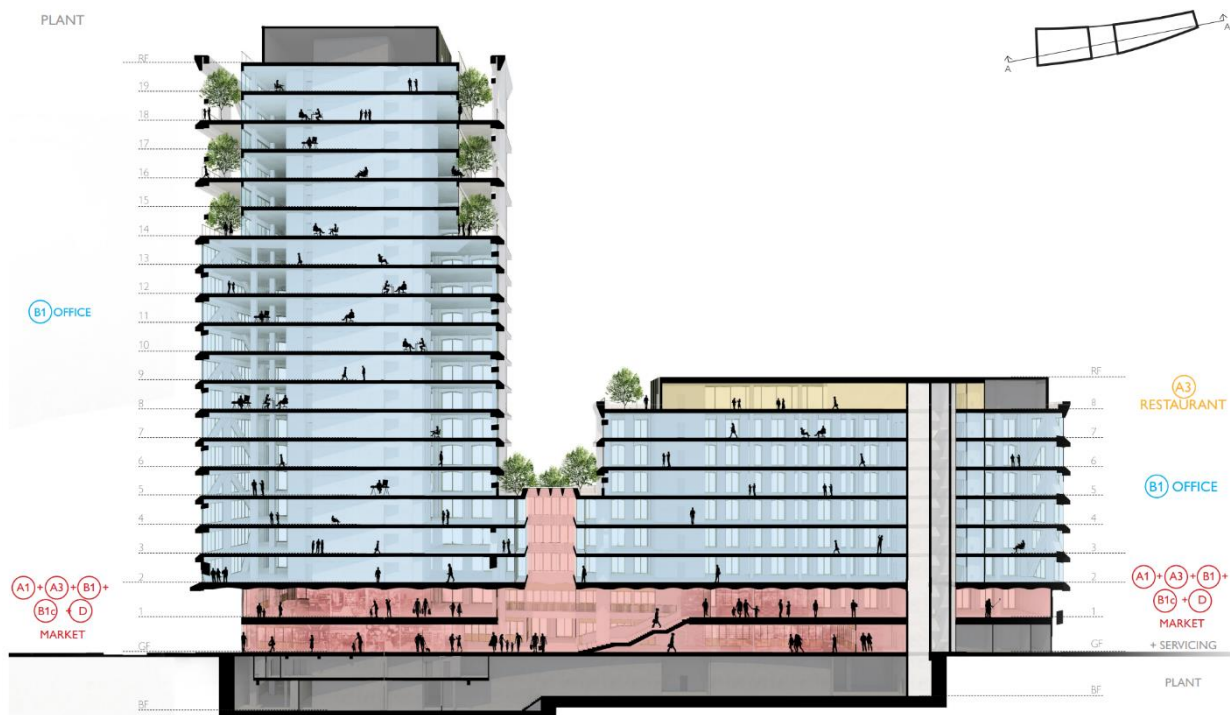
Figure 6 – Cross-section showing proposed uses by floor (Blue: office space, Red: internal retail/market and community space; Yellow: restaurant, Grey: plant, servicing and basement) [Image from DAS addendum July 2020].
