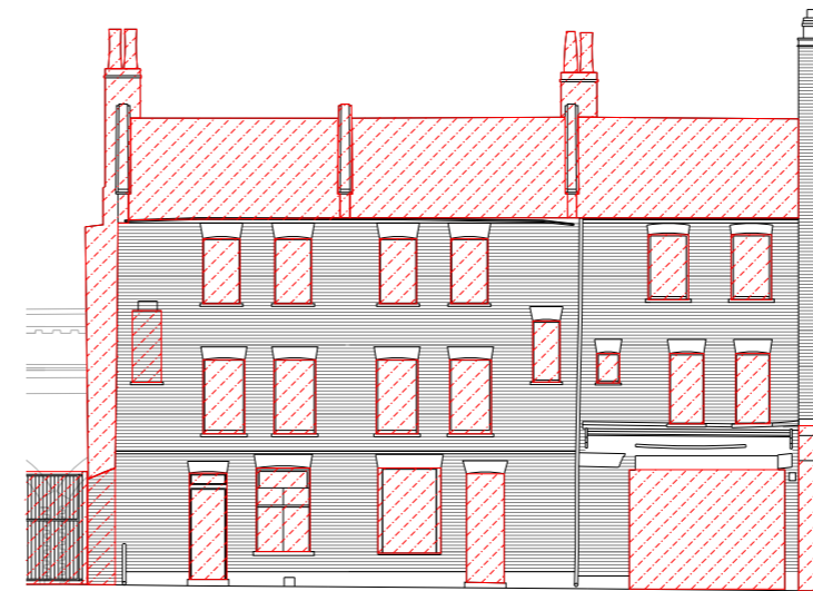
Weavers Cottages. Front - Retained Facade
