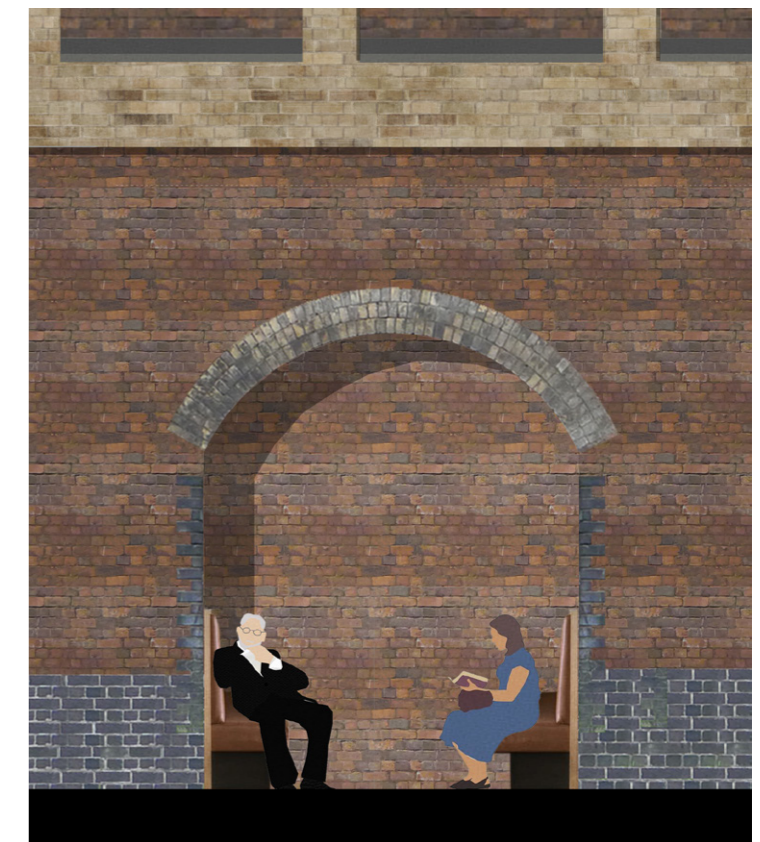
Arch type E - Infill panel to the rear of the arch in brick to match existing, creating a nook.
