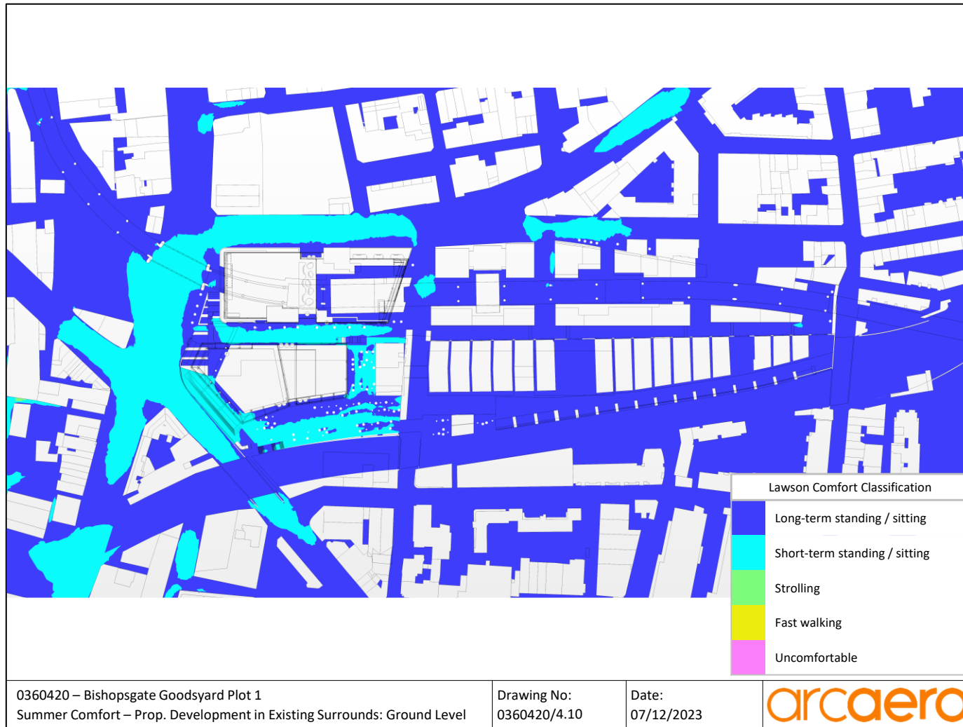
Figure 4.10 Pedestrian wind conditions, proposed development within existing surrounds, summer season – ground level
