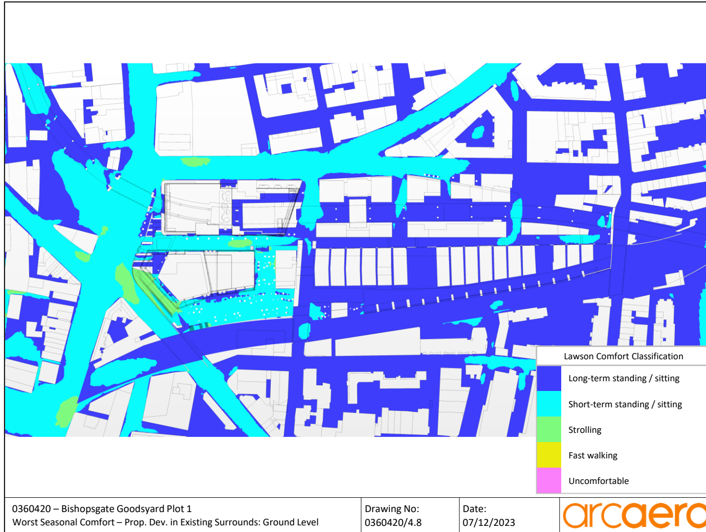
Figure 4.8 Pedestrian wind conditions, proposed development within existing surrounds, worst case season – ground level
