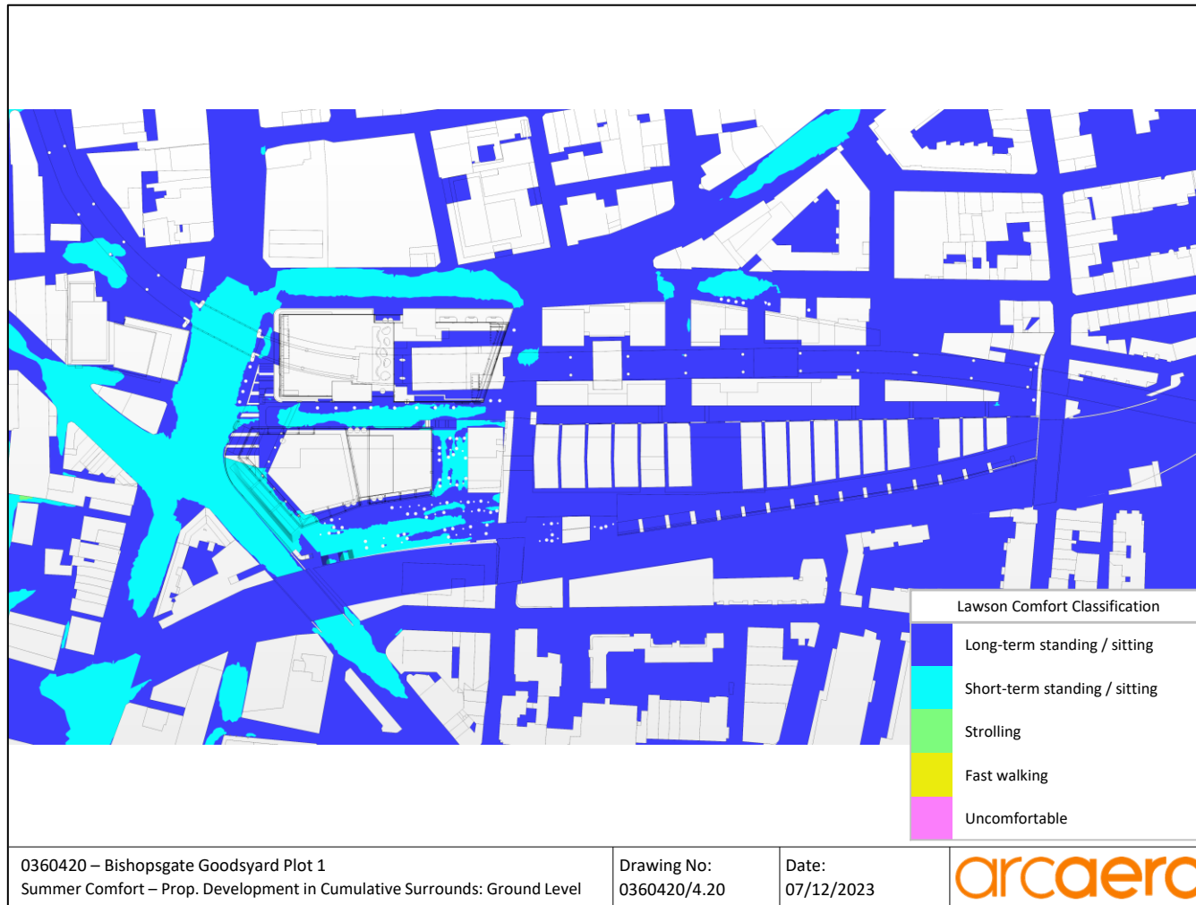
Figure 4.20 Pedestrian wind conditions, proposed development within cumulative surrounds, summer season – ground level
