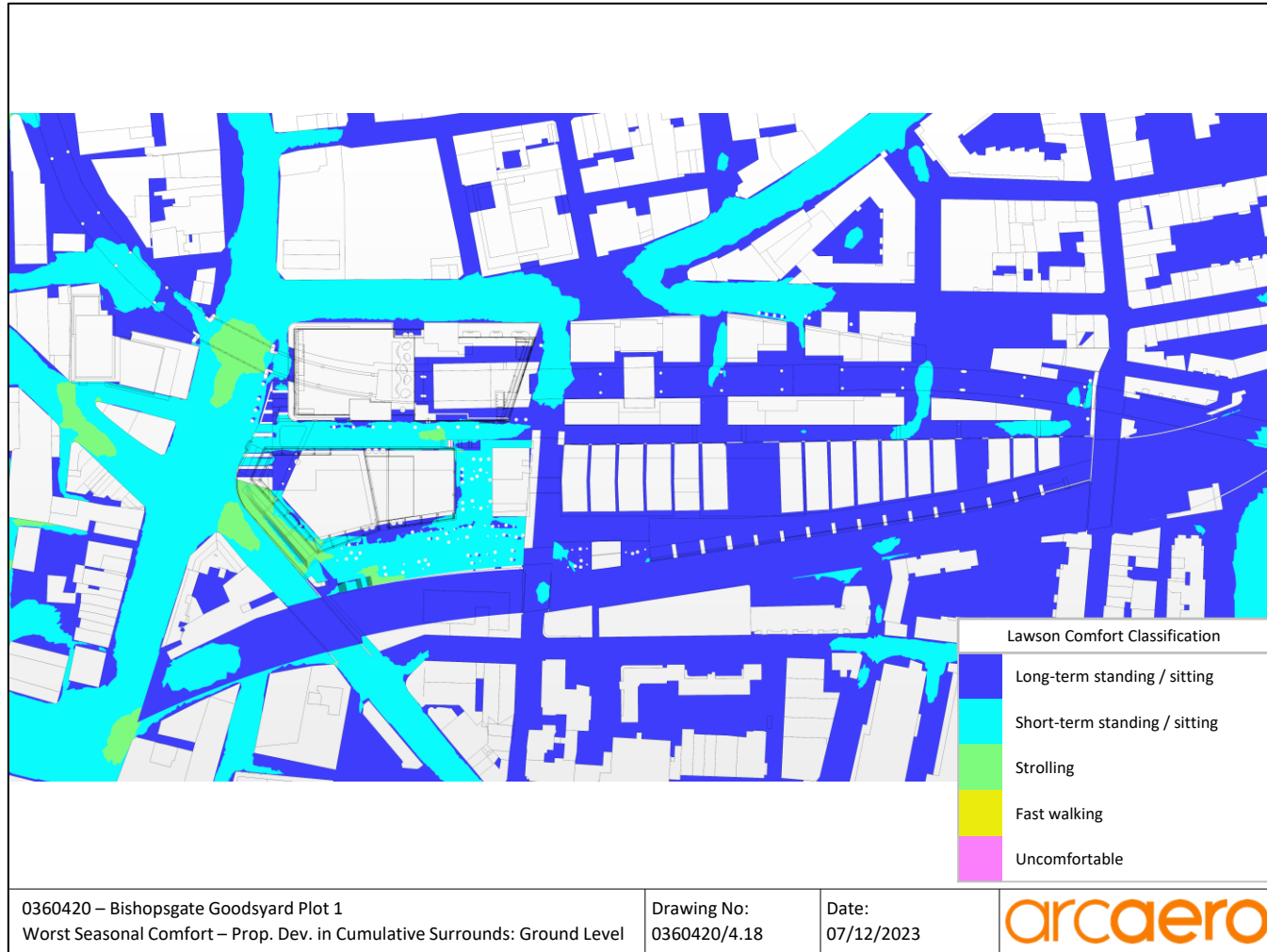
Figure 4.18 Pedestrian wind conditions, proposed development within cumulative surrounds, worst case season – ground level
