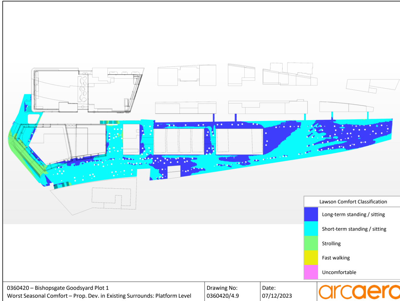
Figure 4.9 Pedestrian wind conditions, proposed development within existing surrounds, worst case season – platform level
