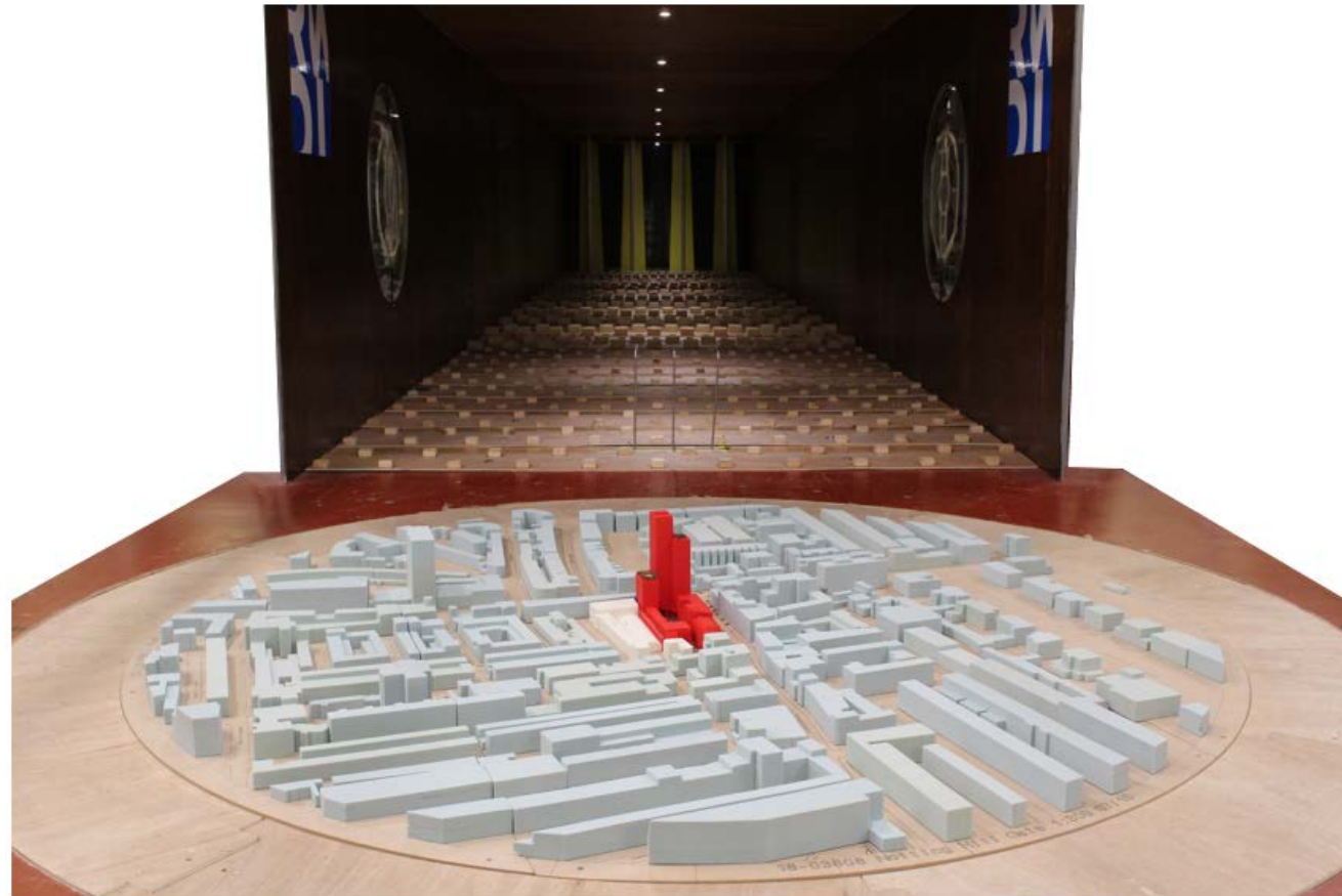
Figure 19: The Proposed Development with existing surrounds (Configuration 1) – View in the Wind Tunnel (from the South)
