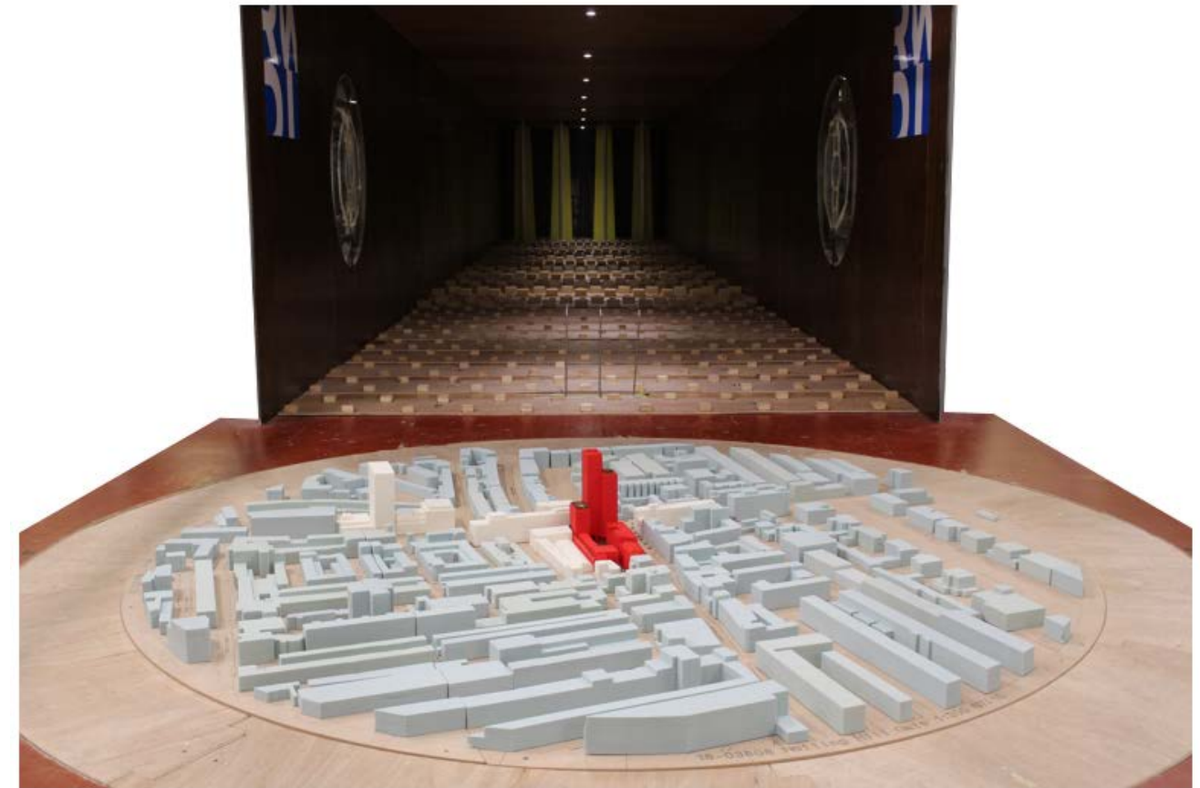
Figure 20: The Proposed Development with cumulative surrounding buildings (Configuration 2) – View in the Wind Tunnel (from the South)
