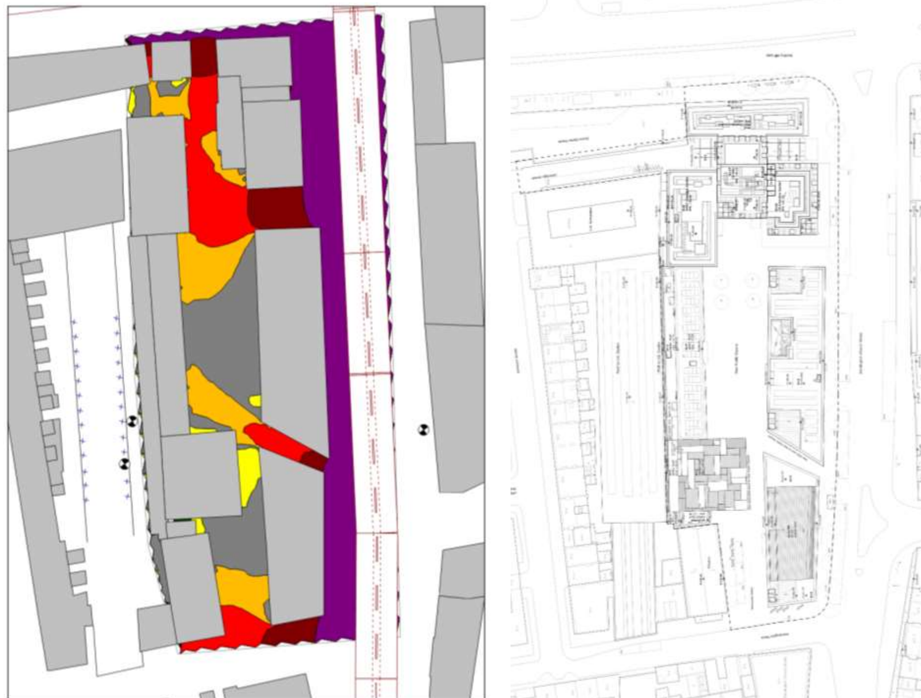
Figure 3: CADNA Noise Map of Proposed Development during the Daytime ( L_{Aeq,16hr} ) at 1.5m height
