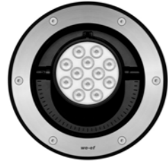
A. In-ground uplights focused towards feature arches Narrow to wide beam recommended interchangeable optics to be provided. Adjustable. 3000K.
