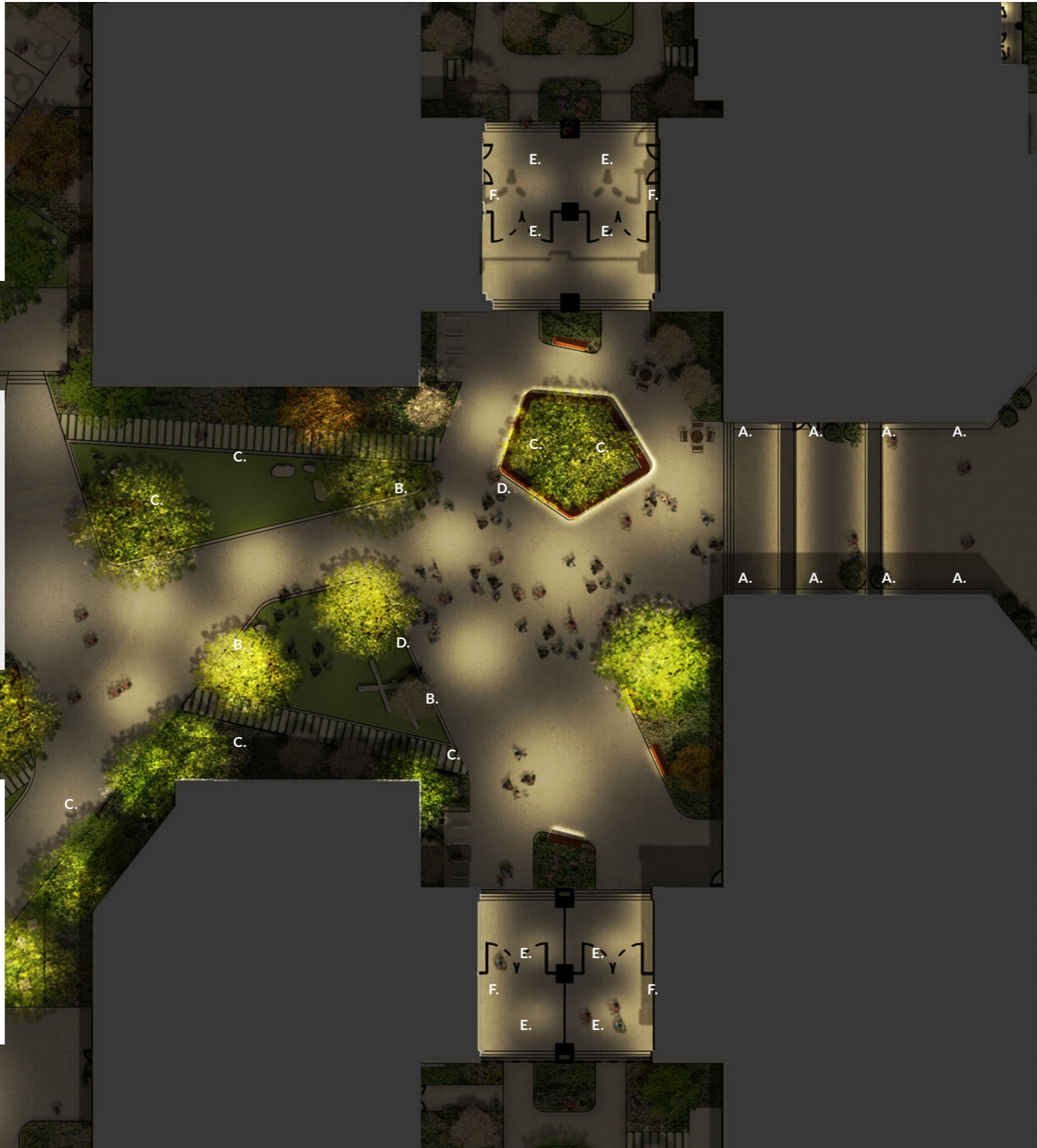
D. Homogeneous Linear LED to be concealed within landscape elements High IP and IK rating required. 3000K.
