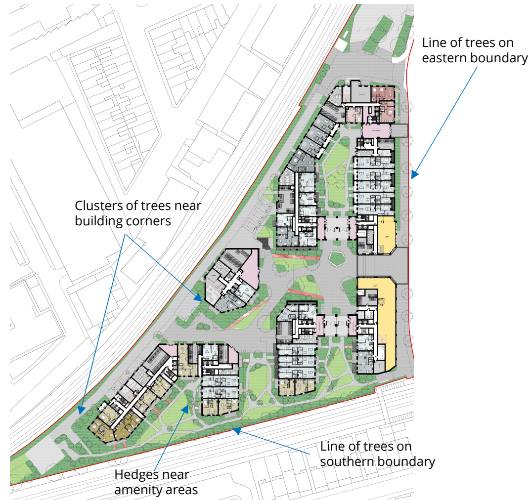
Figure 10: Landscape plan with elements incorporated for improving wind conditions around the blocks.
