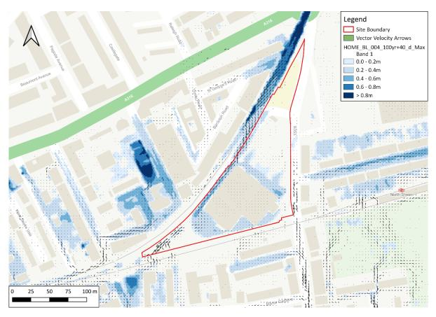
Figure 6. Baseline Modelling - 1 in 100-year plus 40% Climate Change Maximum Depths and Velocity
