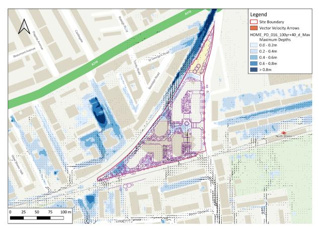
Figure 7. Proposed Development Modelling - 1 in 100-year plus 40% Climate Change Maximum Depths and Velocity
