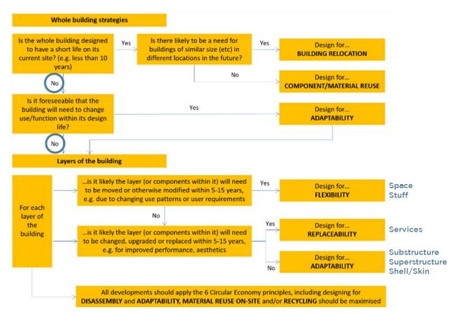
Figure 4-2 - Decision tree for design approaches for new buildings, infrastructure, and layers over the lifetime
