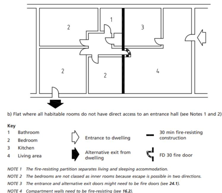
Figure 3 Flats provided with alternative means of escape from bedroom
