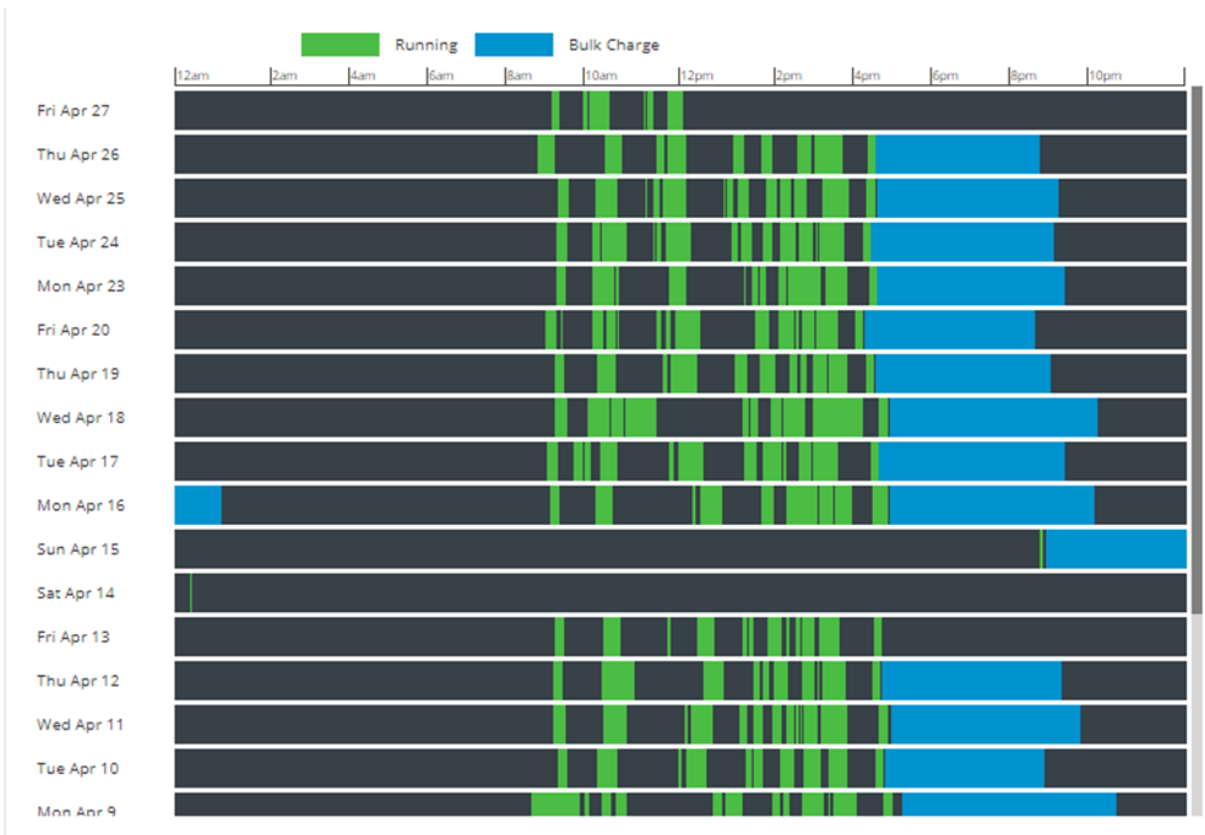
Figure 3: Typical EV charging routine where green is times when the vehicle is driven and blue when it is being charged
