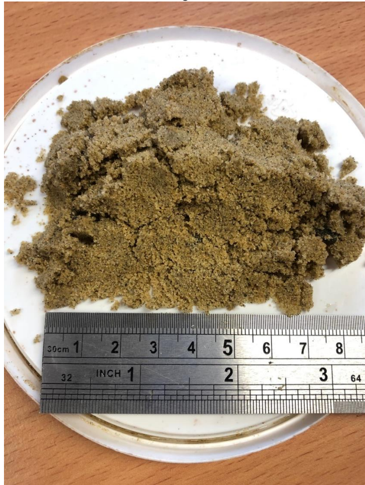
Sand discharged from BH2
