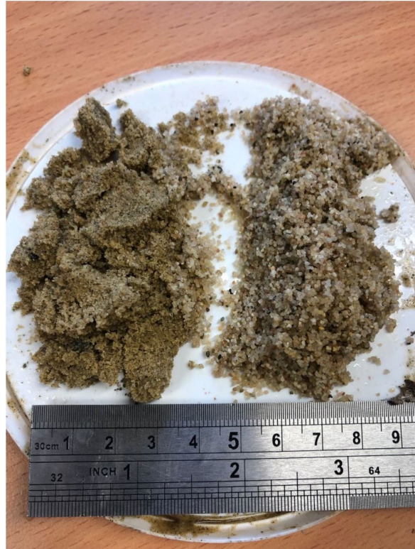
Comparison of sand discharged from BH2 (left) with a 0.5 mm to 1.0mm graded sand (right)
