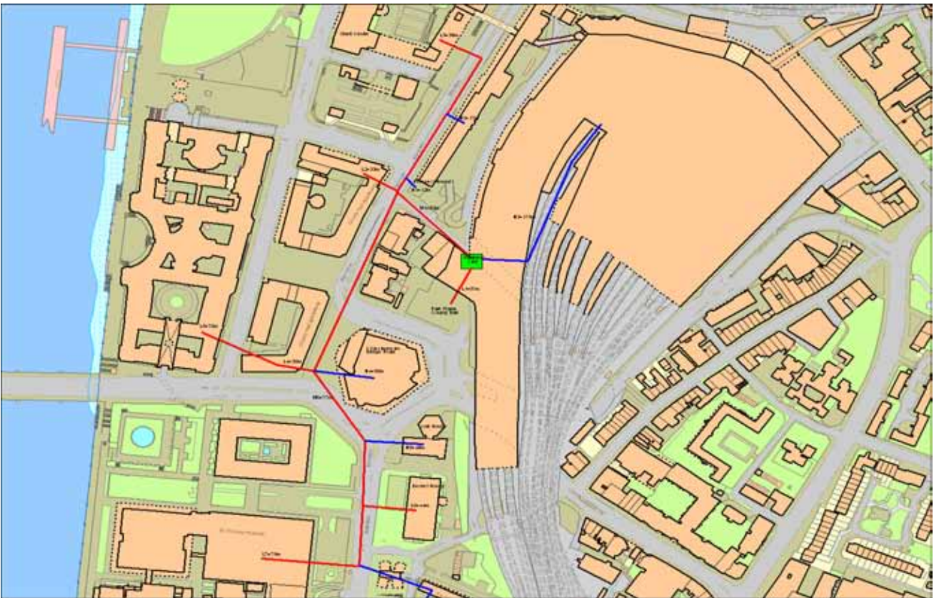
Figure 6.12 Waterloo cluster pipework (Estimated pipework cost - £2.0m)
