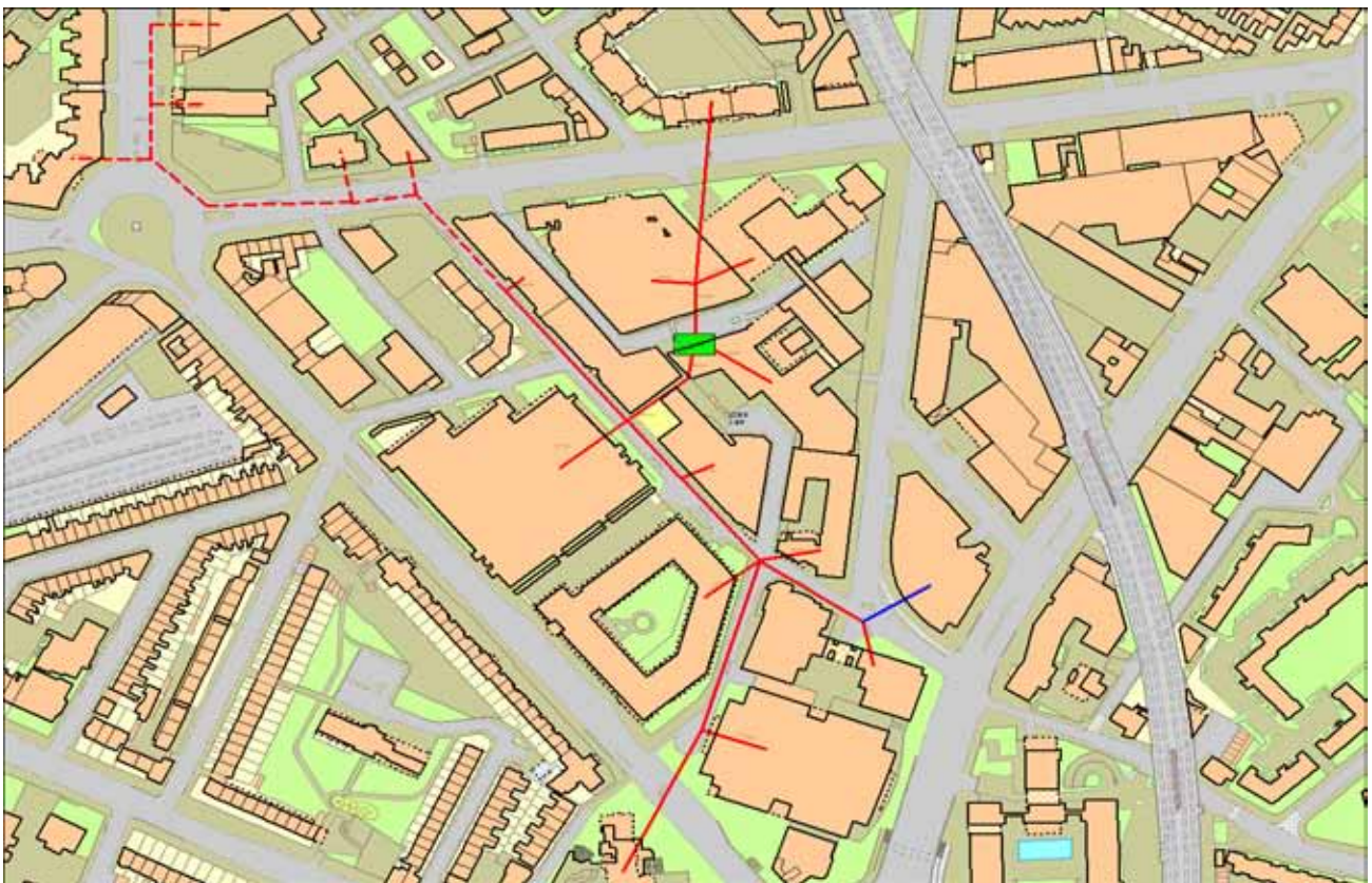
Figure 6.10 LSBU cluster pipework (Estimated pipework cost - £0.7m exc dotted, Maclaren House test)
