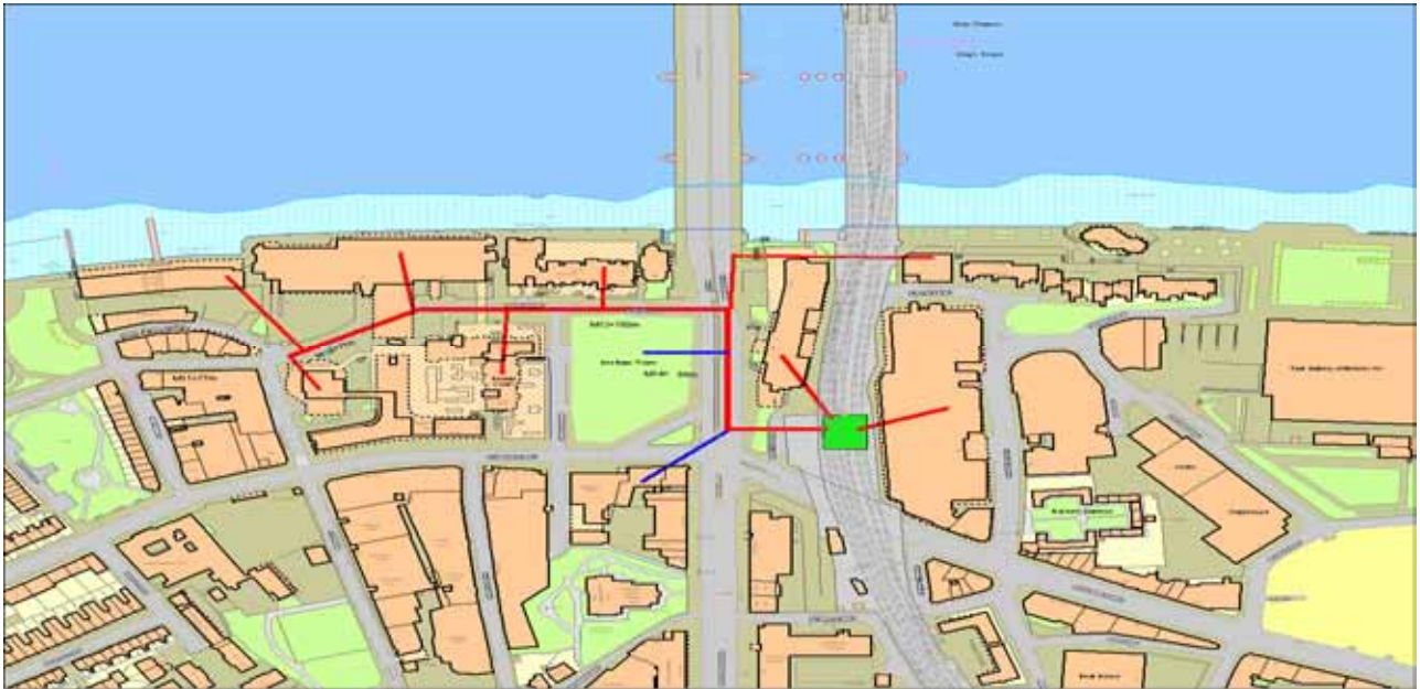
Figure 6.9 Blackfriars cluster pipework (Estimated pipework cost ~ £0.98m)
