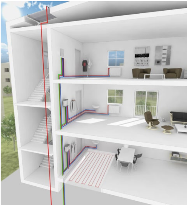
Figure 21: Image of heat interface units installed in an example consumer building (courtesy of Danfoss).
