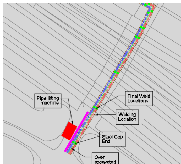
Figure 39 Installation method - north end
