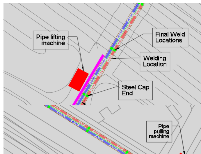
Figure 38 Installation method - south end
