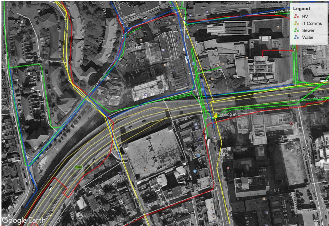
Figure 3-28 - Utility mapping nr Wandle Rd Energy Centre
