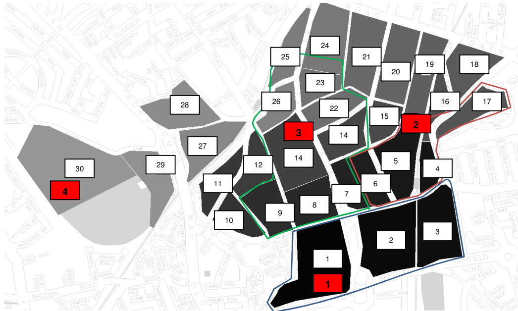
Figure 6 Proposed locations of the Zonal Energy Centres and an indication of the Energy Clusters they will serve respectively
