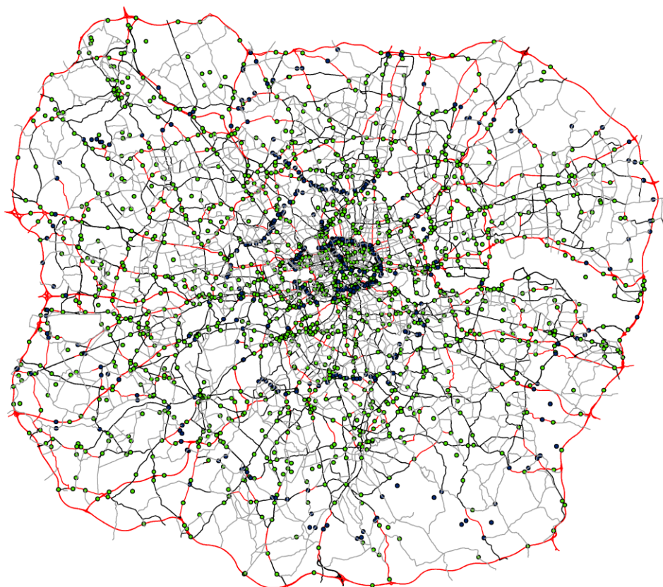
Figure 2 The LAEI 2013 road network. Major road links are in black, LTS road links are in grey. Circles represent the manual classified count (MCC) sites used to determine major road traffic; green circles are for DfT count sites and navy ones for TfL. Major road links updated with 2013 data are highlighted in red.
