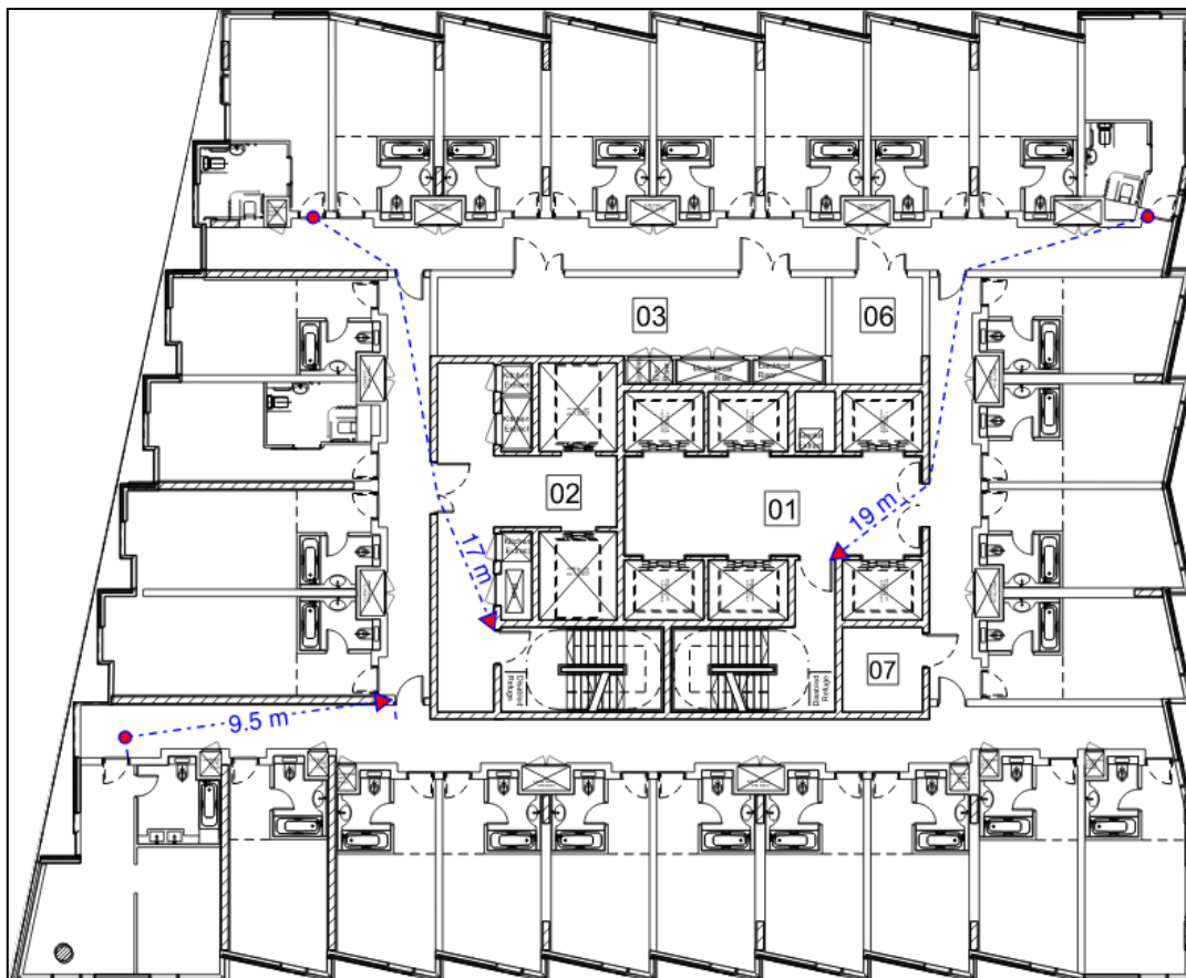
Figure 2 - North Tower Escape Distance
