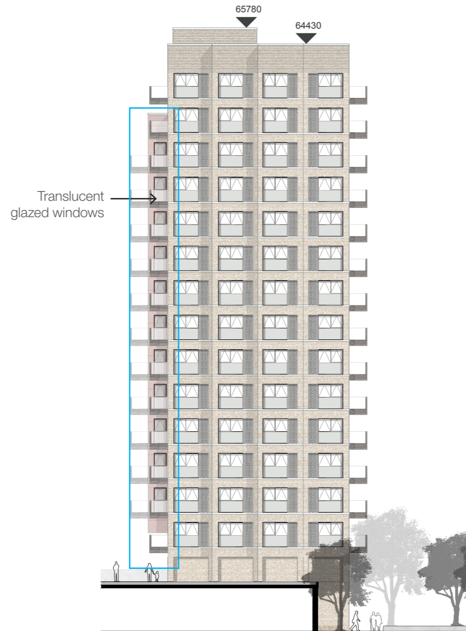
Elevation showing the new windows to the north facing return wall on Core 1.
