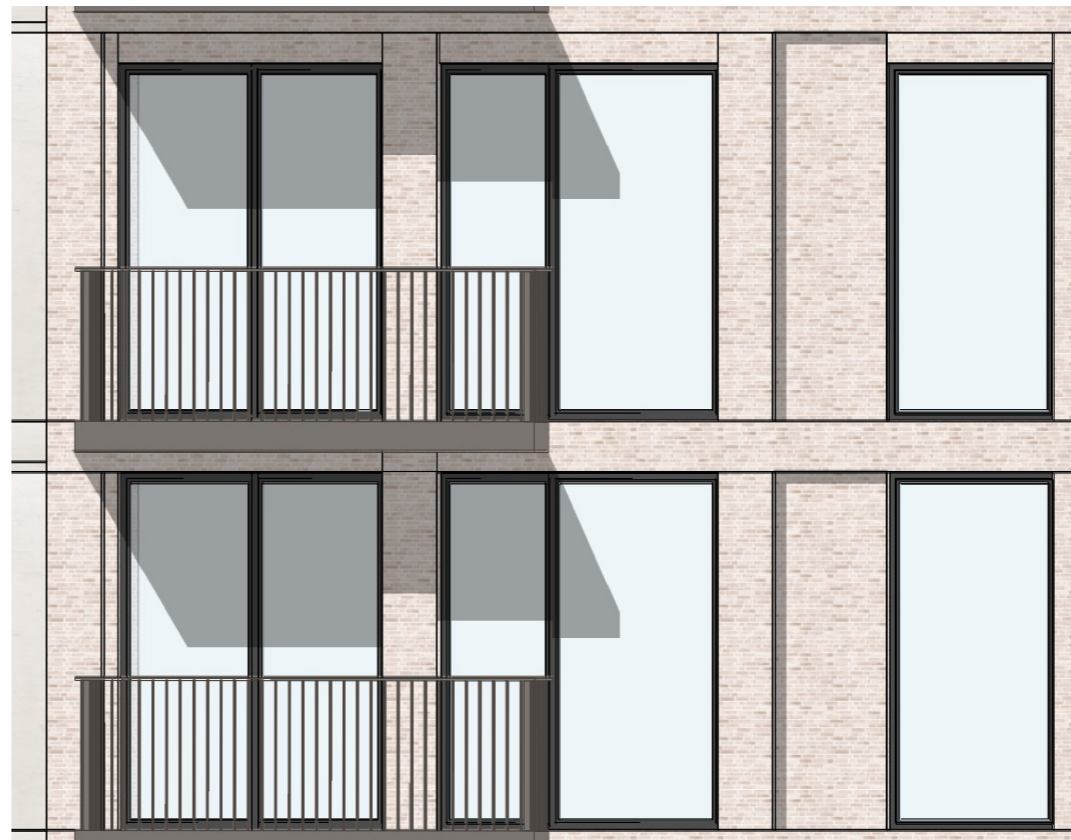
Building C_west facade_additional window
