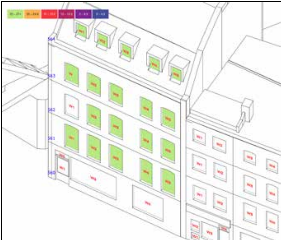
Existing VSC Levels (196 Shoreditch High Street)
