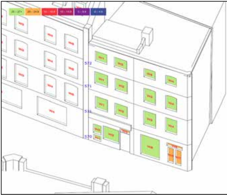
Existing VSC Levels (194 – 195 Shoreditch High Street)
