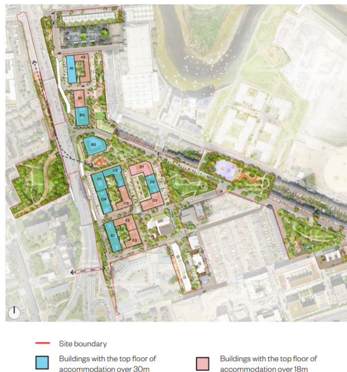
Figure 15: Proposed illustrative masterplan (excluding detailed phases) showing buildings with the top floor of the accommodation over 18 metres in height shown in a terracotta-coloured overlay, and the buildings with the top floor of the accommodation over 30 metres in height shown in the blue overlay.
