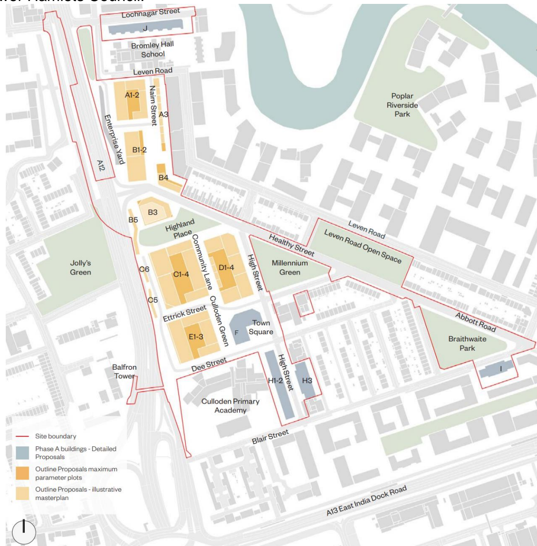
Figure 7: Layout of proposed development plots, as originally submitted to Tower Hamlets Council. Diagram also illustrates the relationship between the maximum parameters and the illustrative masterplan (Source: Original Masterplan DAS).
