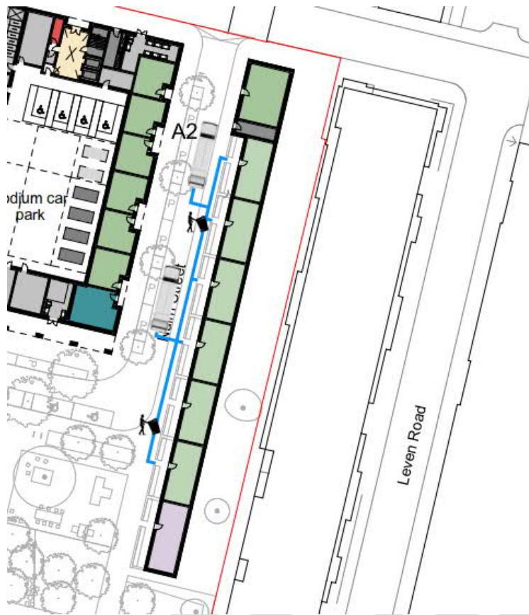
Figure 5-4 RCV Loading Position Plot B4 on Abbott Road (Illustrative Scheme)
