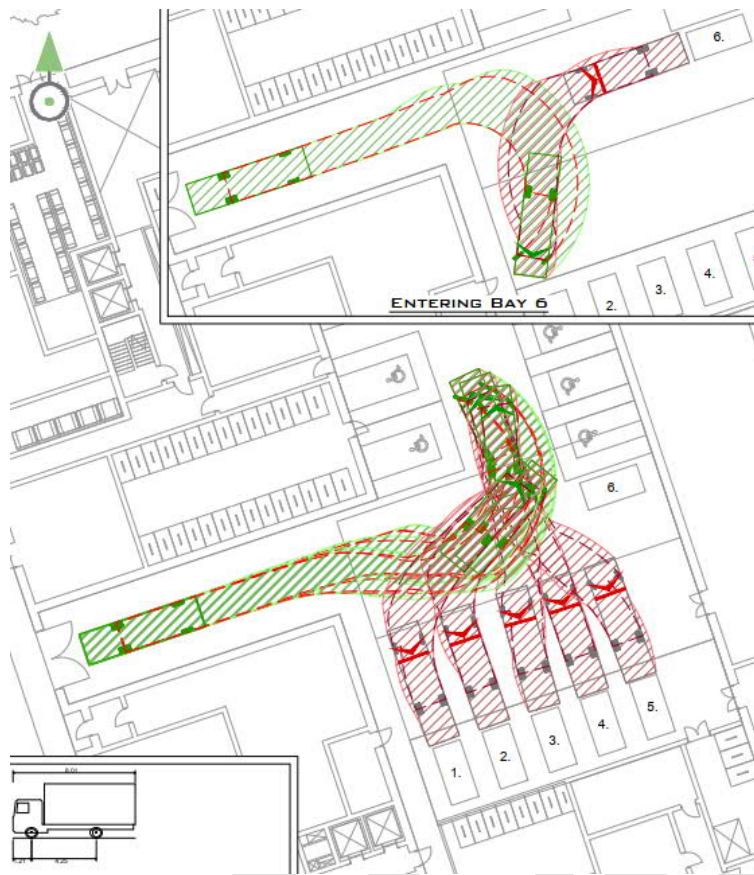
Figure 5-15 Plot E Compactor Collection (Illustrative Scheme)
