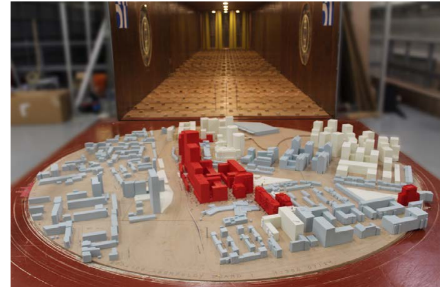
Fig.774 View of the illustrative massing with Cumulative Surrounding Buildings in the wind tunnel
