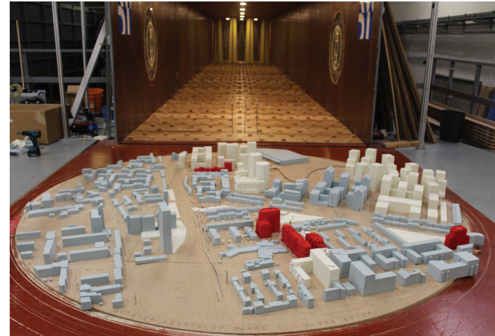
Figure 23: Detailed Proposals (Phase A) with Cumulative Surrounding Buildings (Configuration 7, Board 1) – View in the Wind Tunnel (from the south)
