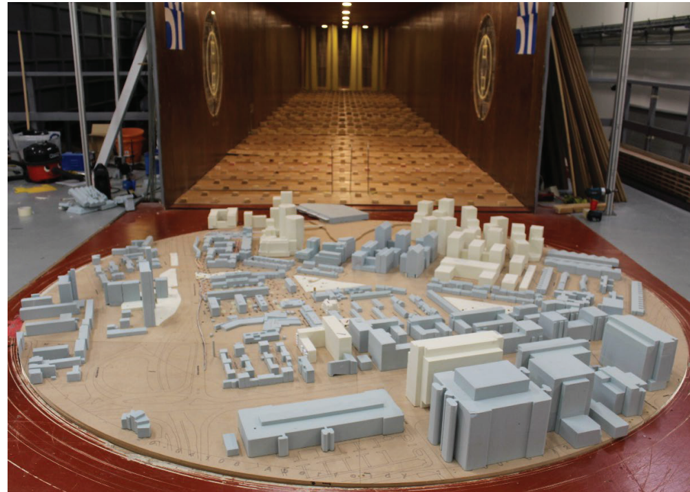
Figure 21: Existing Site with Cumulative Surrounding Buildings (Configuration 6, Board 2) – View in the Wind Tunnel (from the south)
