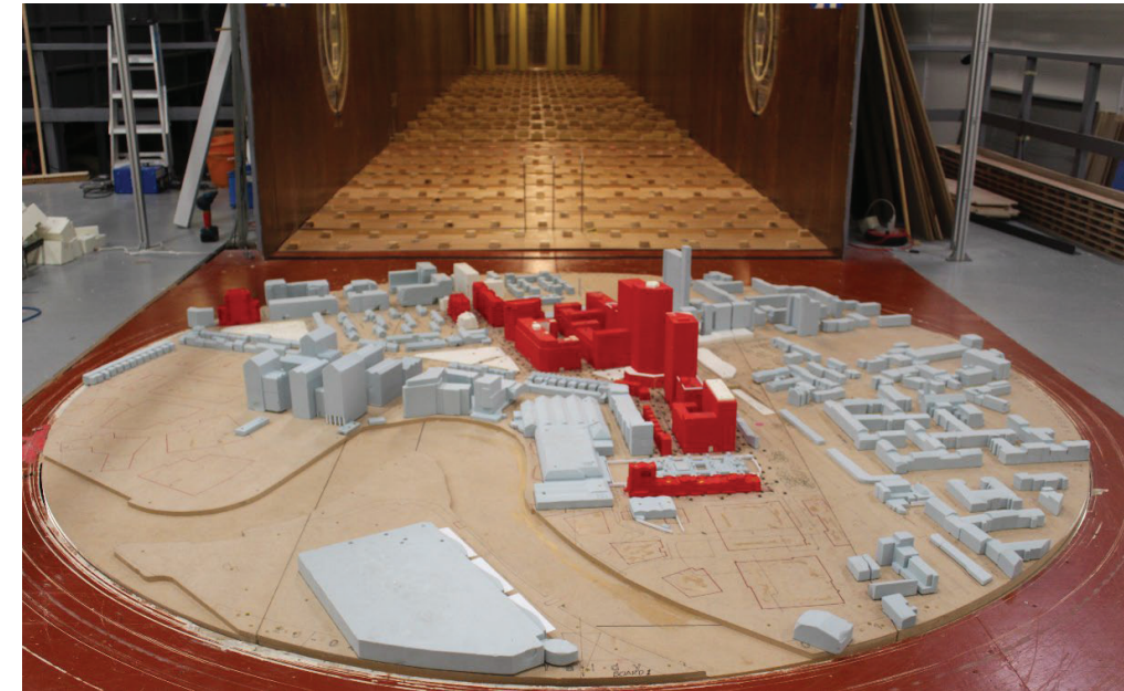
Figure 15: Proposed Development (Illustrative Scheme) and Phase A with Existing Surrounding Buildings (Configuration 4, Board 1) – View in the Wind Tunnel (from the north)
