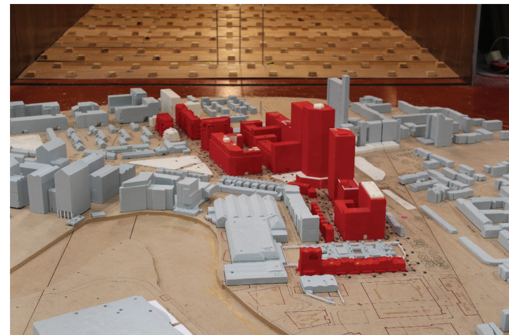
Figure 16: Proposed Development (Illustrative Scheme) and Phase A with Existing Surrounding Buildings (Configuration 4, Board 1) – View in the Wind Tunnel (from the north)
