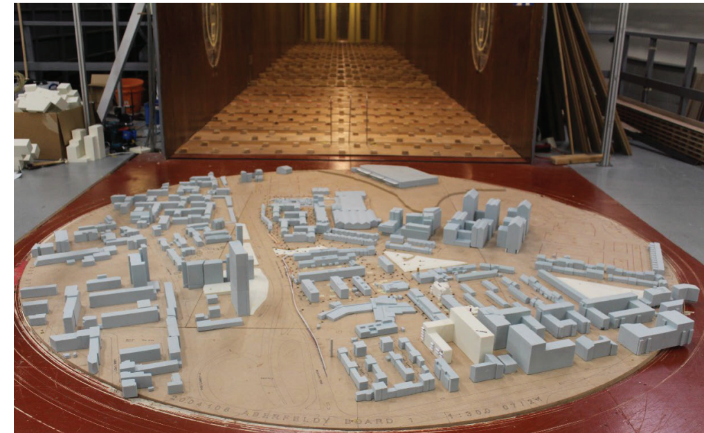
Figure 3: Existing Site with Existing Surrounding Buildings (Configuration 1, Board 1) – View in the Wind Tunnel (from the south)
