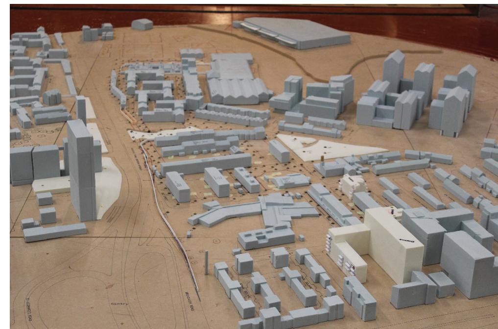
Figure 4: Existing Site with Existing Surrounding Buildings (Configuration 1, Board 1) – View in the Wind Tunnel (from the south)
