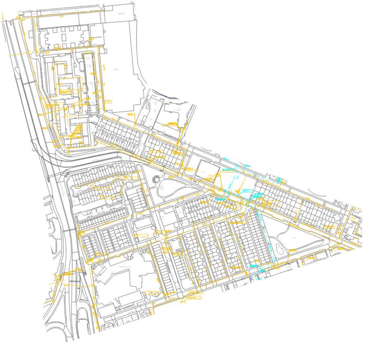
Figure 8: Existing Gas Services Asset Plan
