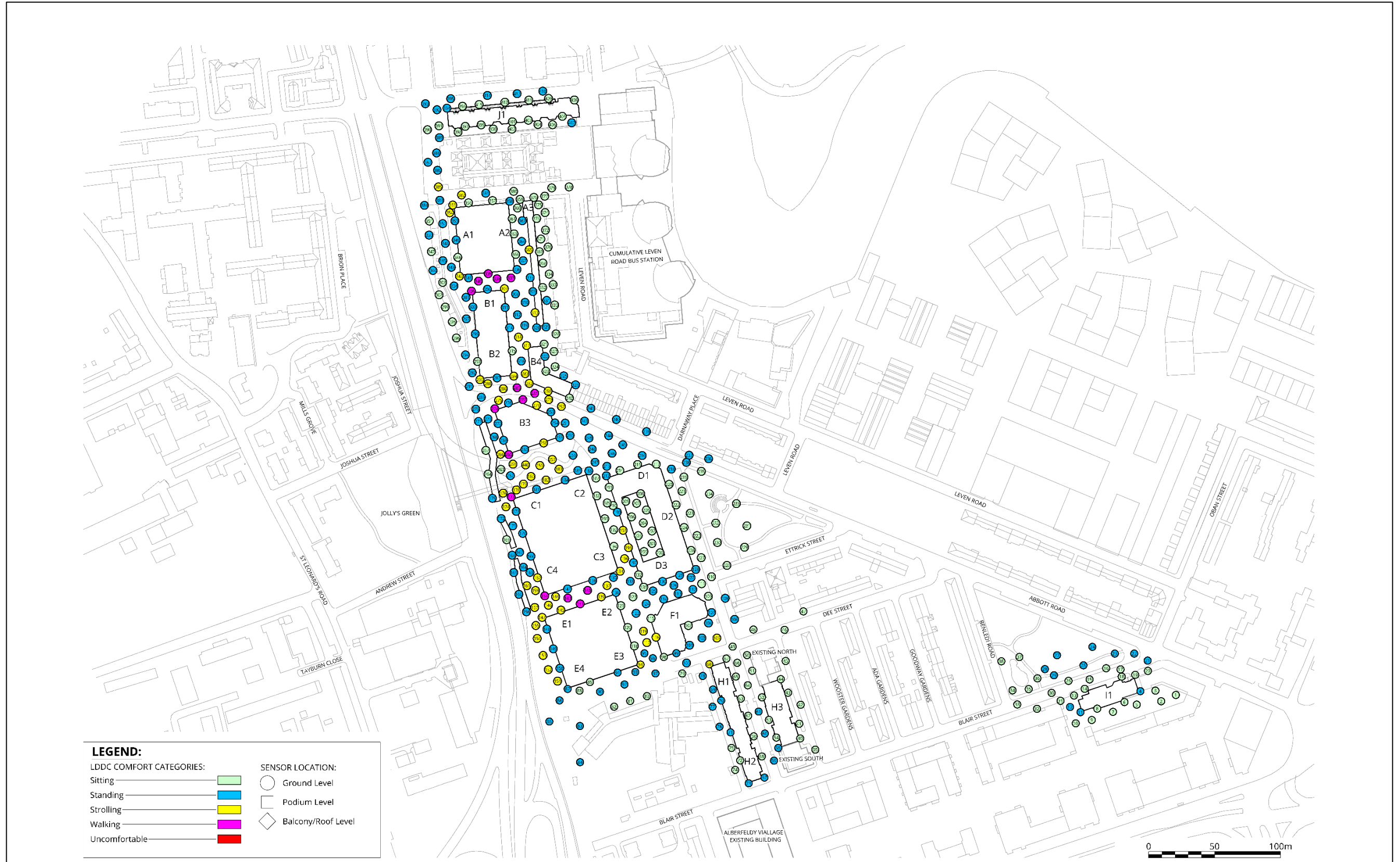
Figure 13.46 Configuration 8: Proposed Development (Outline Proposals plus Detailed Proposals) with Cumulative Surrounding Buildings – Ground Level (Windiest Season)
