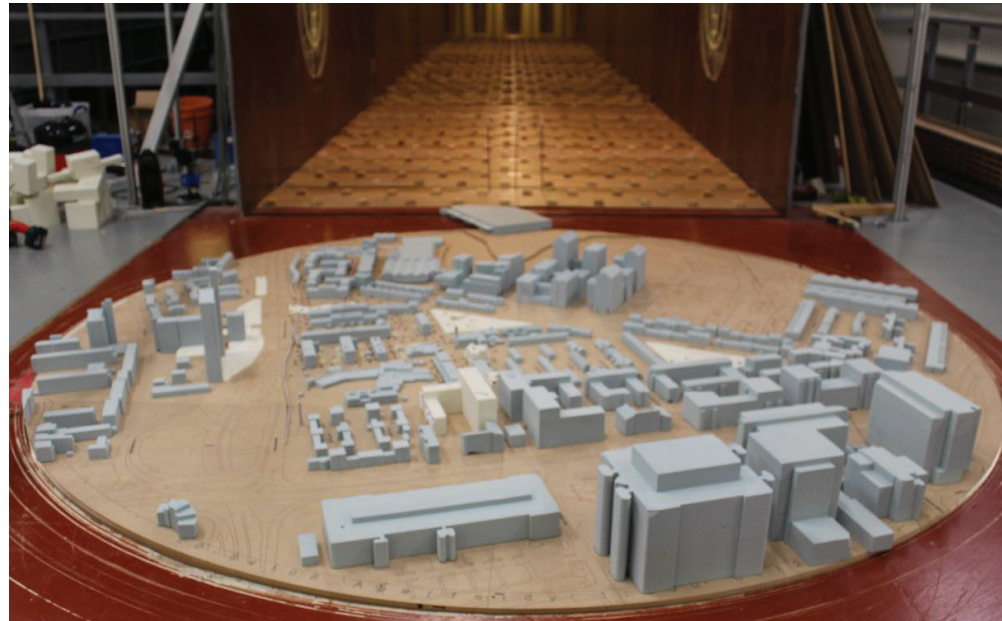
Figure 5: Existing Site with Existing Surrounding Buildings (Configuration 1, Board 2) – View in the Wind Tunnel (from the south)
