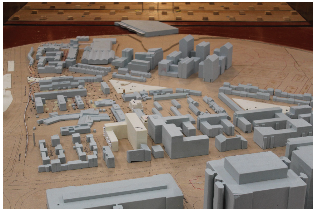
Figure 6: Existing Site with Existing Surrounding Buildings (Configuration 1, Board 2) – View in the Wind Tunnel (from the south)
