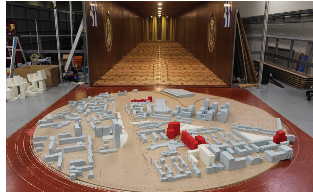
Figure 7: Detailed Proposals (Phase A) with Existing Surrounding Buildings (Configuration 2, Board 1) – View in the Wind Tunnel (from the south)
